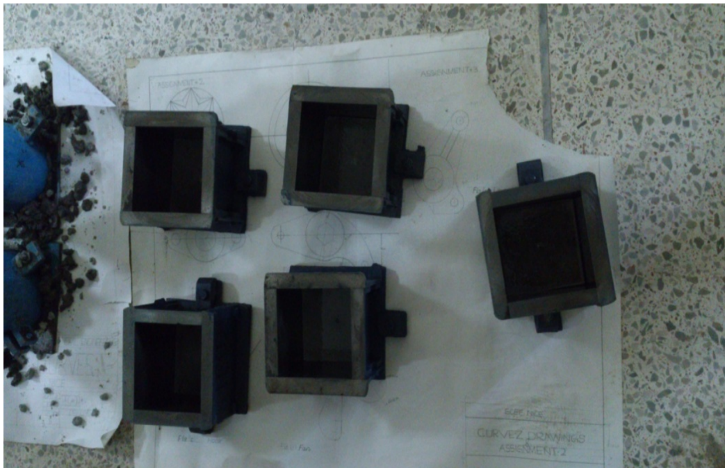
Figure 5: Molds; Oiled and Ready for Casting
