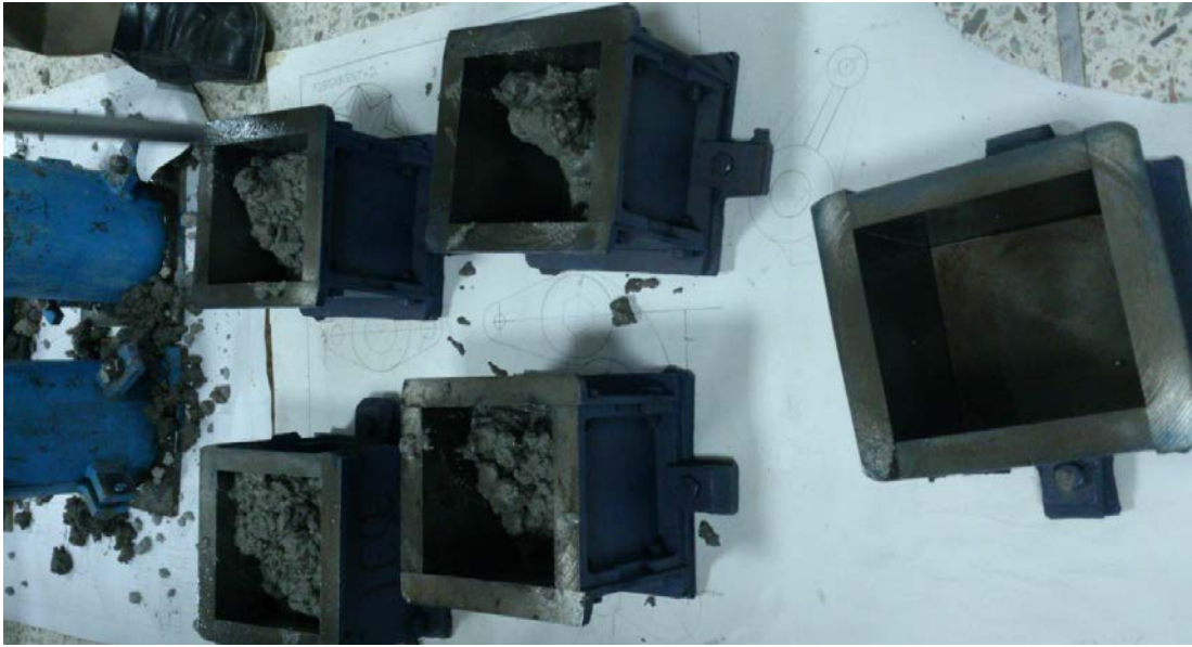
Figure 6: Molds; Being Filled with Concrete Mix
