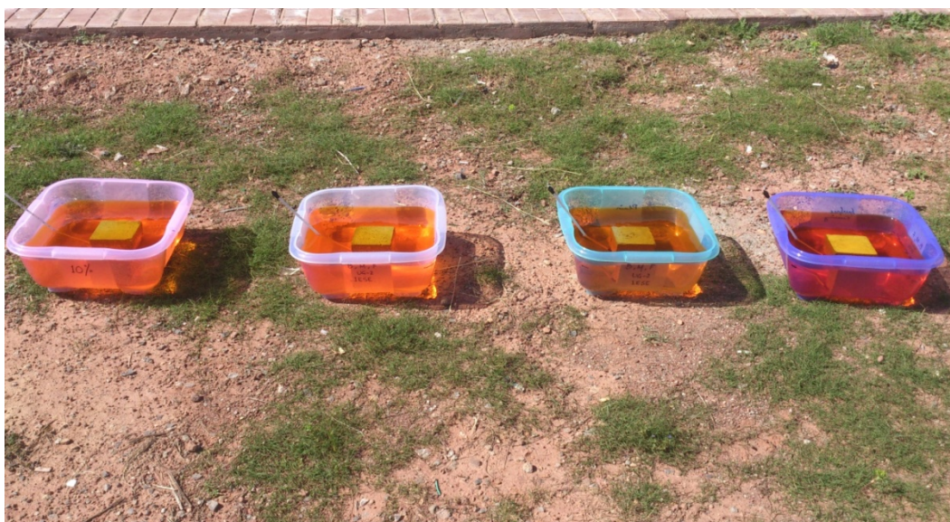
Figure 18: Concrete Blocks Testing With Methyl Orange
