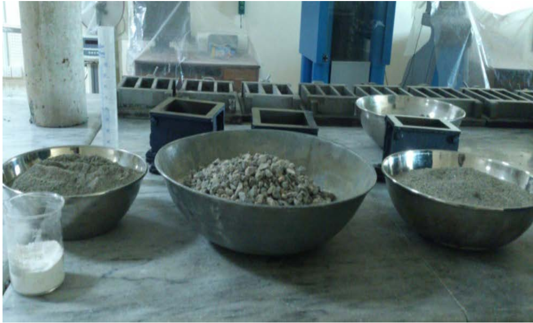
Figure 4: Cement, Coarse Aggregate, Fine Aggregate, TiO 2 Nanoparticles, Water and Molds
