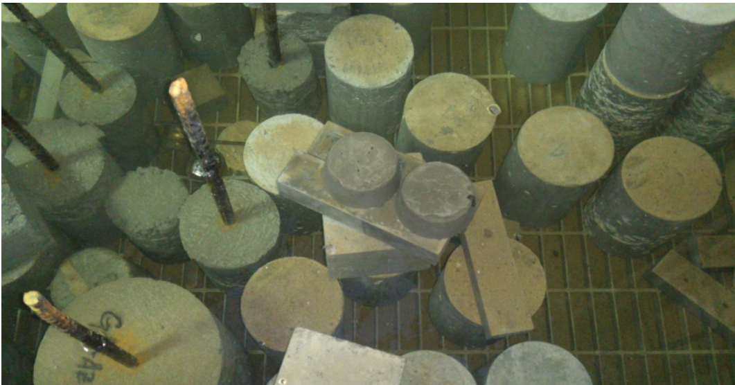
Figure 11: Curing of Concrete Blocks
