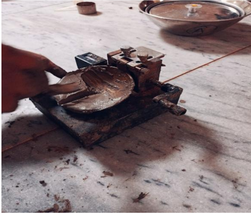
Figure 3.5 Casagrande method for Atterberg's limit
