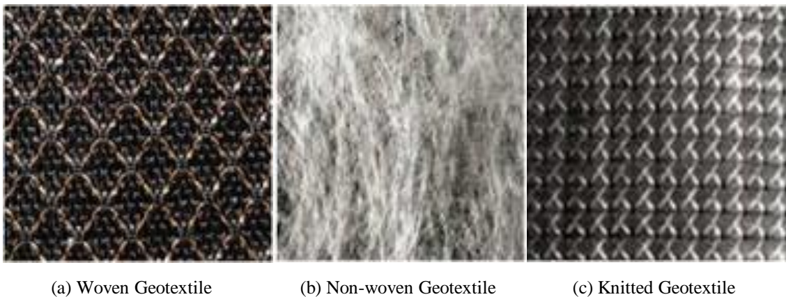
Figure 1.1 Different geotextile; (a) woven geotextile, (b) non-woven geotextile and (c) knitted geotextile
