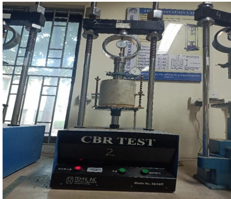
Figure 3.8 CBR Test performed on reinforced soil sample
