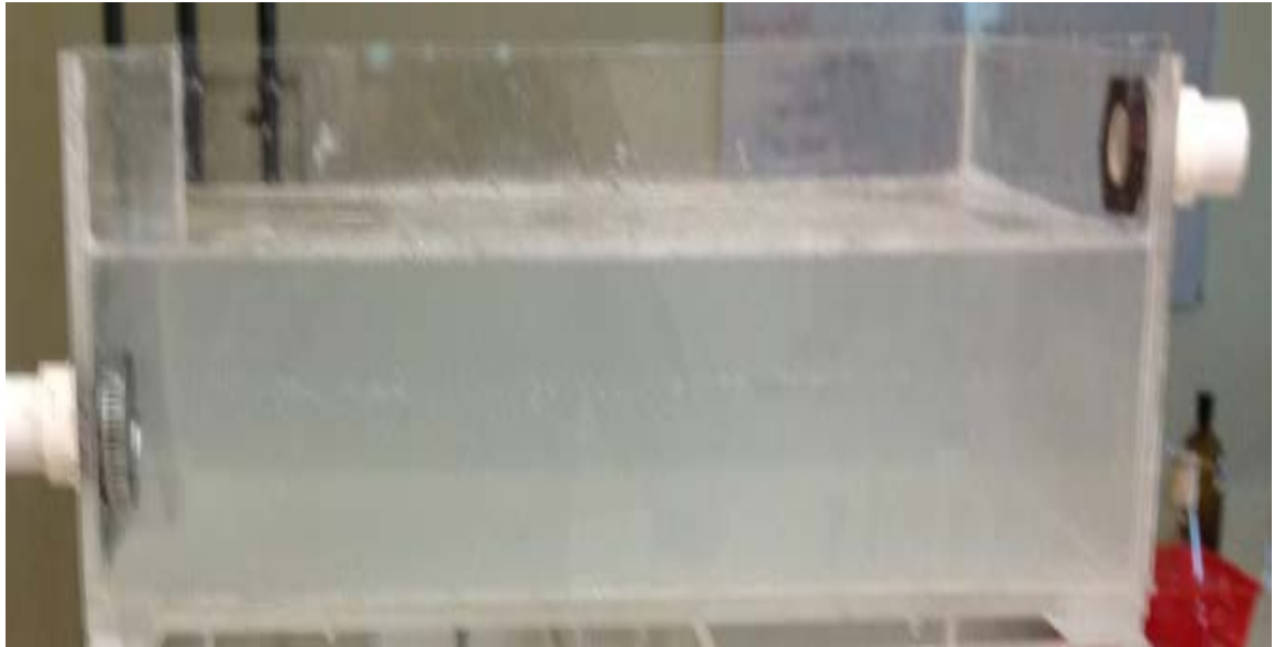
Figure 10 Sedimentation/ Collection Tank
