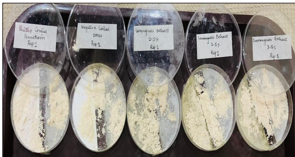
Figure 3.8: Experimental Setup for Testing % Repellency of Pest Using Different Concentrations of Plant Extracts with reference to Control
