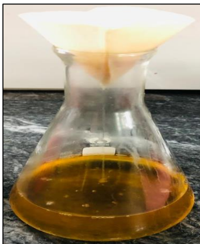
Figure 3.3: Filtration of the extract to separate solid tailings of the plant sample
