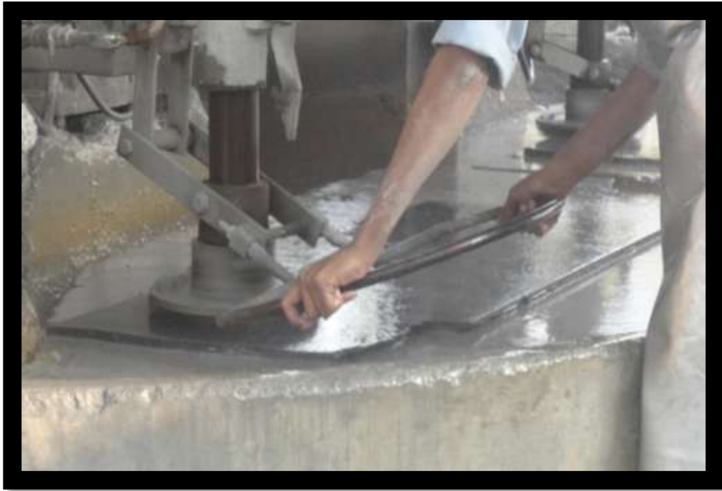
Figure 5: Polishing the marble surface to add shine using water
