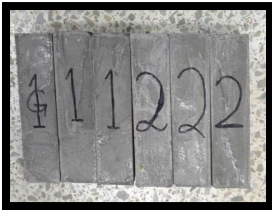
Figure 21: Prisms prepared for compression strength tests
