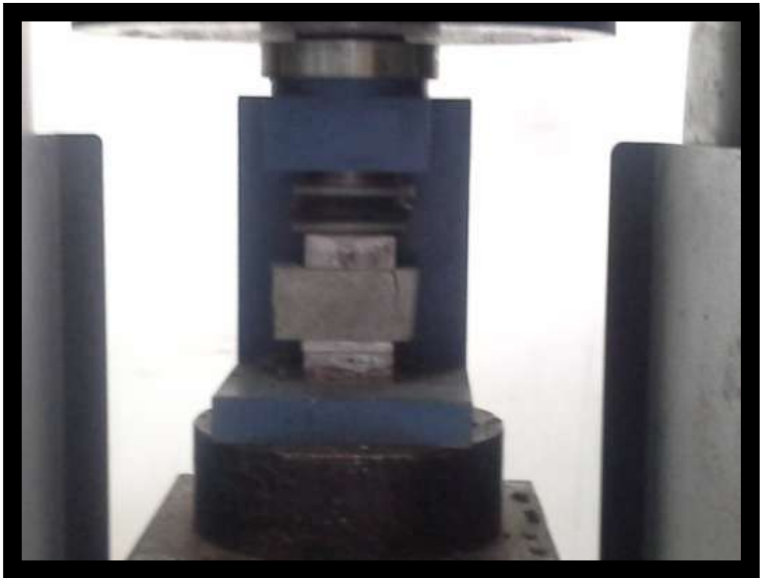
Figure 22: Compressive strength test in UTM machine
