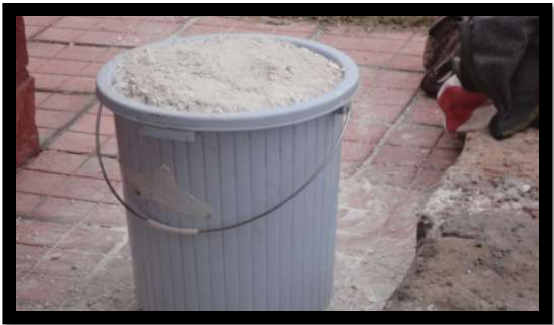
Figure 16: Dried marble powder used for further making bricks and tiles
