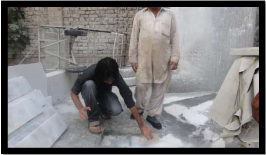
Figure 8: Liquid sample collection after step 2 cutting
