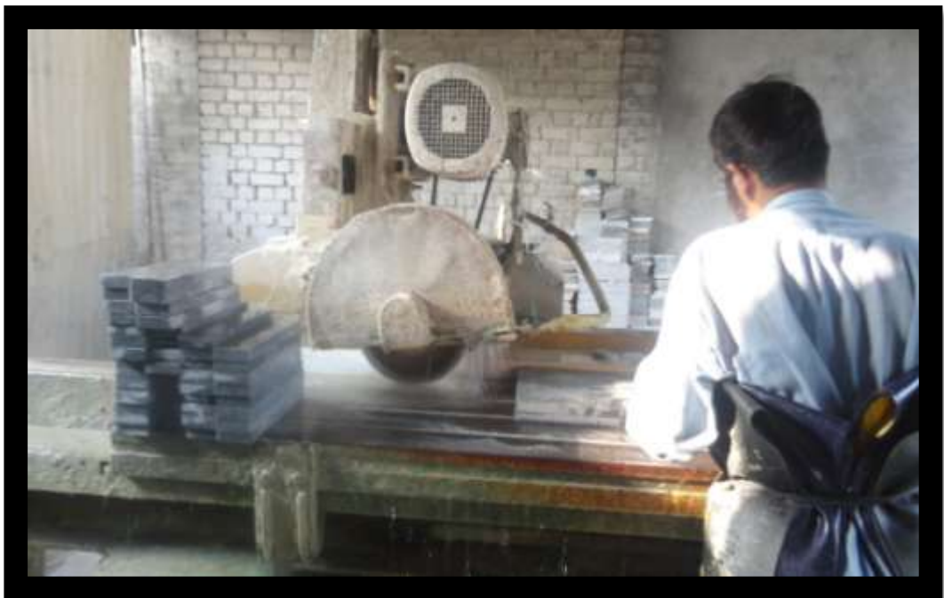
Figure 4: Cutting/sawing into tiles and slabs with spraying water
