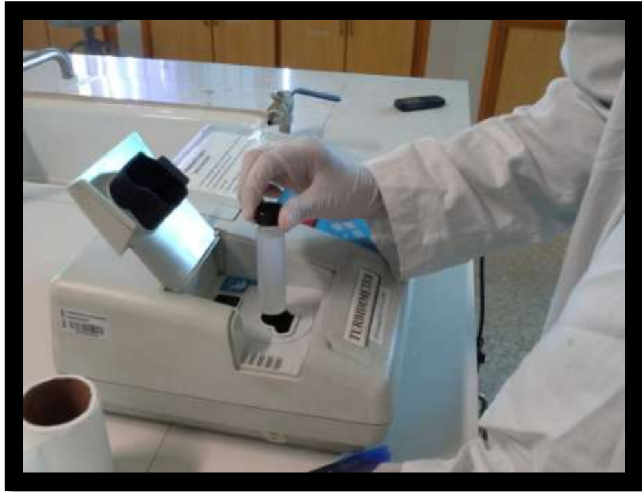
Figure 11: Turbidity meter for measuring the turbidity of effluent
