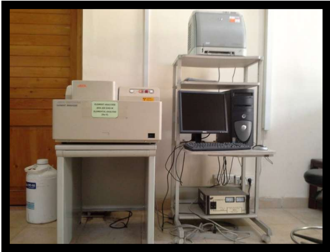
Figure 18: XRF machine used to find chemical composition of the dried samples
