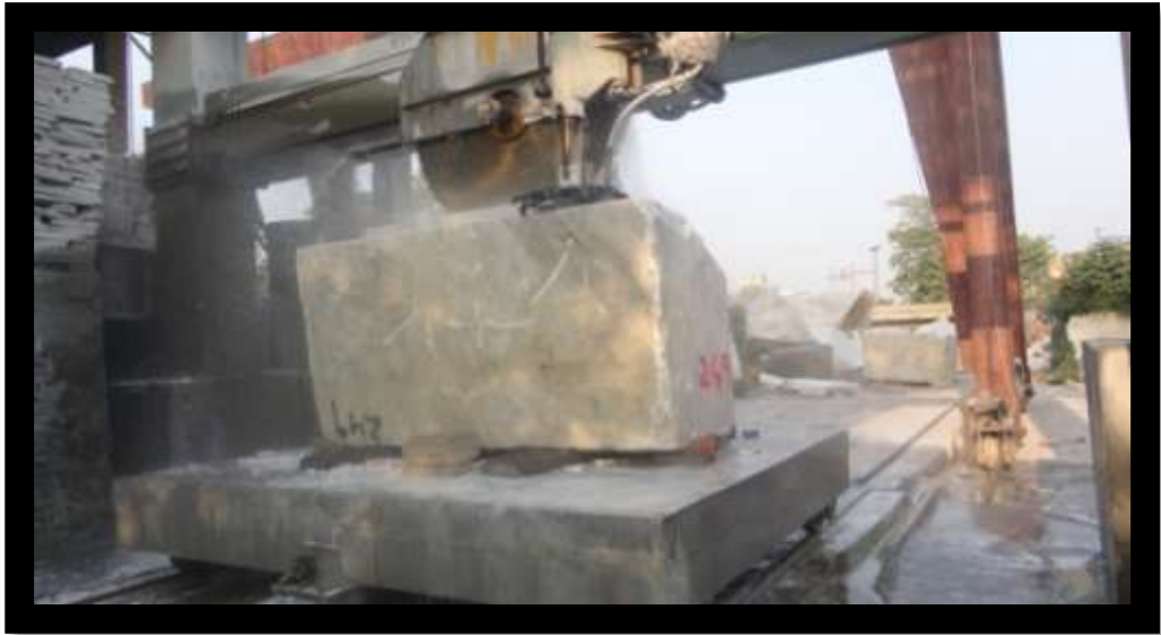
Figure 3: Cutting of large tons into small thickness slabs using large blades and spraying water
