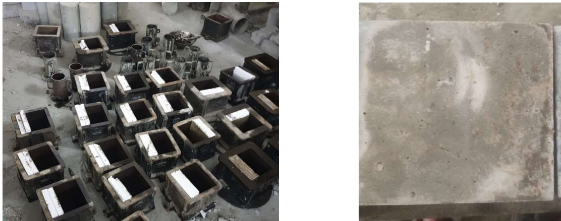
Figure 3.10 Casting of cubes with NSC substrate
