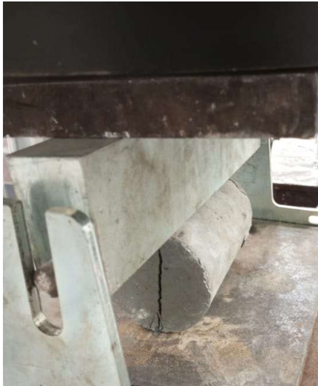
Figure 4.7 Split Tensile Test Assembly
