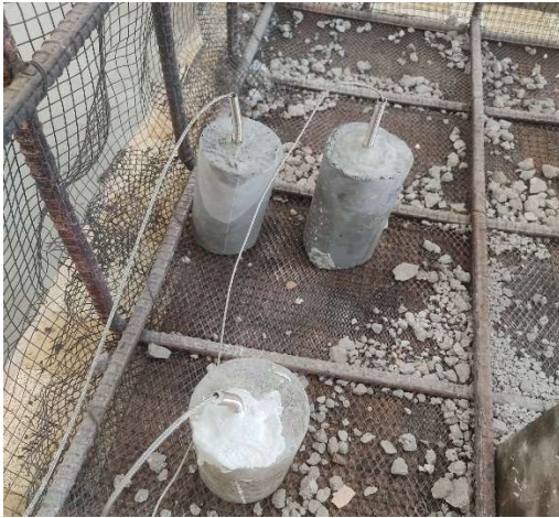
Figure 3.12 Preparation of cylinders to determine rate of heating of core temperature of specimen
