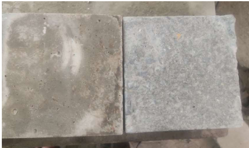
Figure 3.4 Difference between smooth and roughened surface
