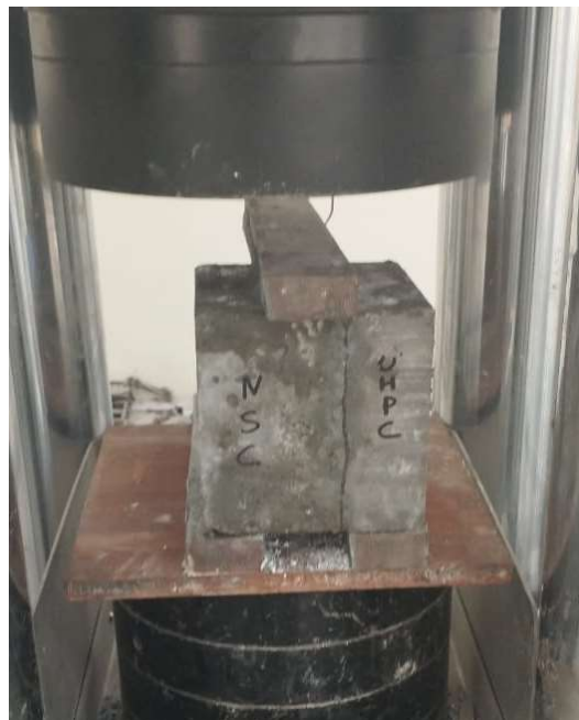
Figure 3.11 Bi-surface shear test setup
