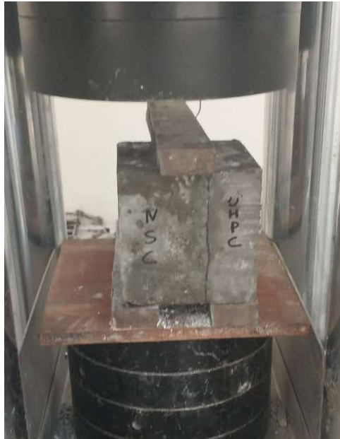
Figure 4.3 Bi-Surface Shear Test Assembly
