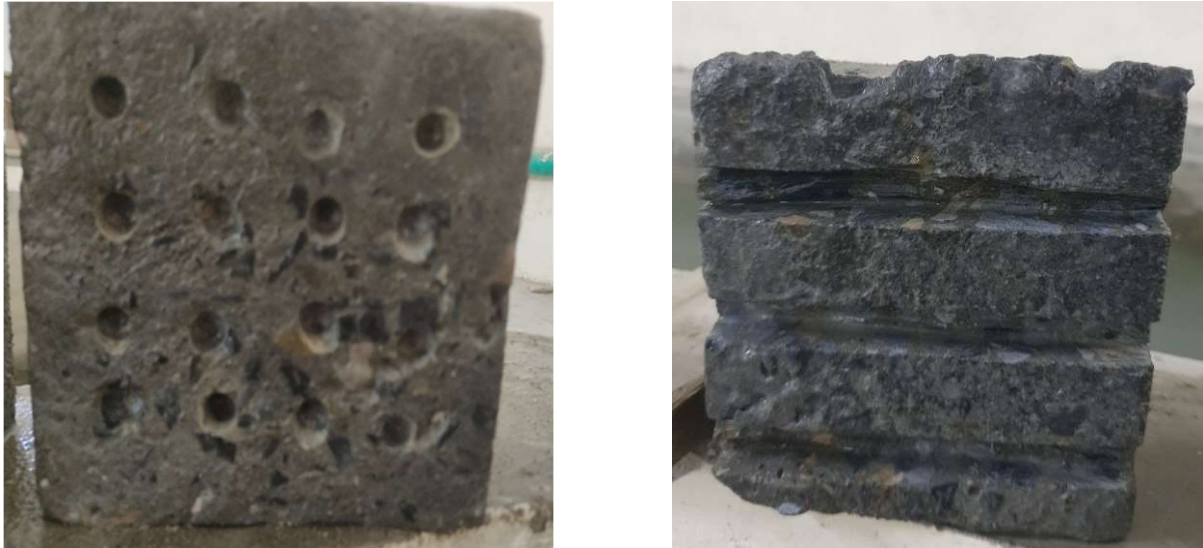
Figure 3.5 Surface preparation of specimen
