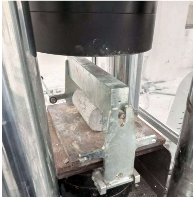
Figure 3.9 Split tensile assembly
