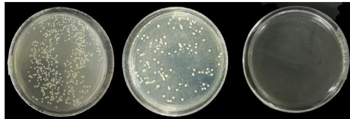
Figure 19: S. mutans growth of unmodified composite resins, composites resin having 1% AgNPs & composite resin having 1% CIP-AgNPs
