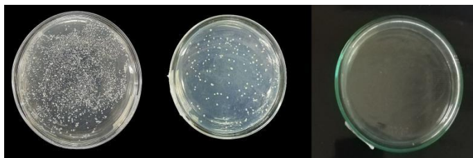
Figure 20: Microcosm bacterial growth of unmodified composite resins, composites resin having 1% AgNPs & composite resin having 1% CIP-AgNPs
