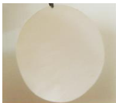
Figure 6: TiO 2 coated membrane.
