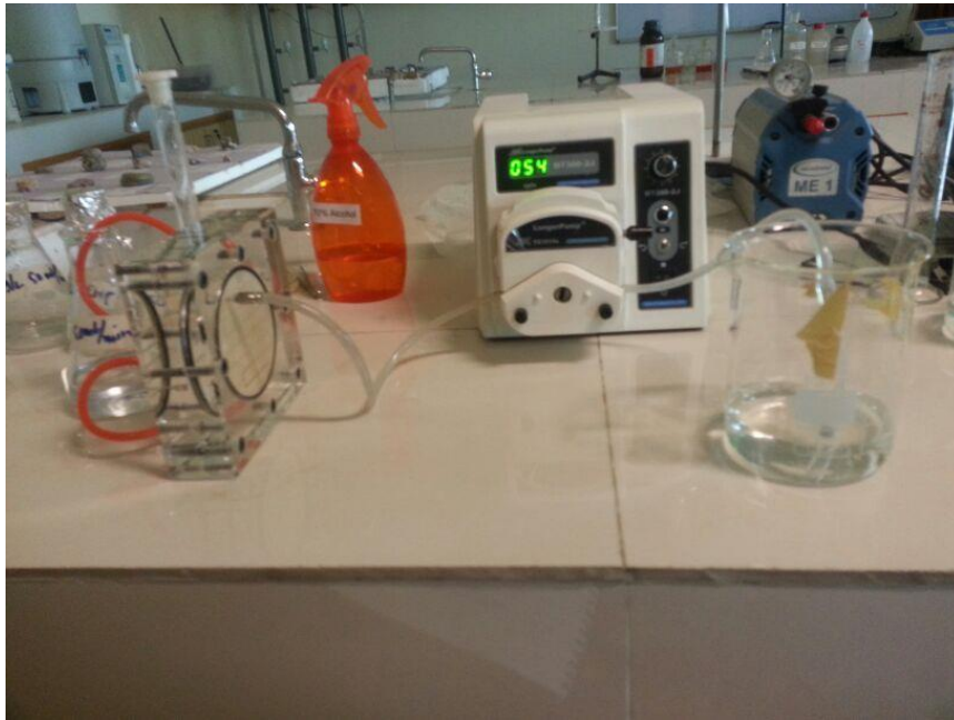
Figure 14: Experimental set up of hybrid filtration system.
