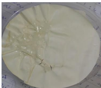
Figure 4: Membrane dipped into pure sol.
