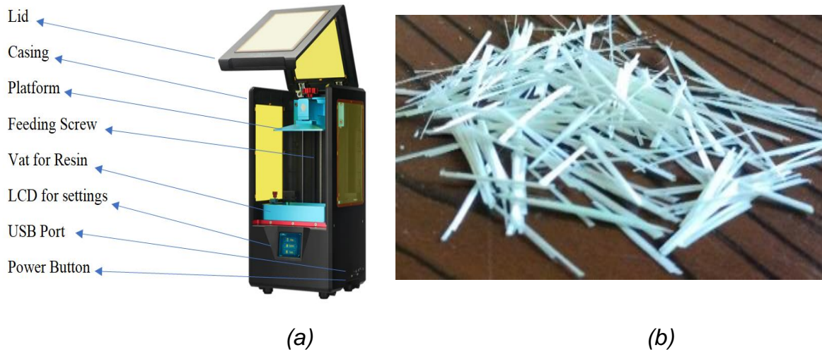
Figure 4 (a) Masked SLA 3d printer (b) Chopped glass fibers
