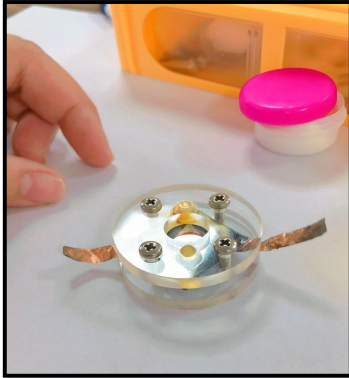
Figure 4.31 Fabricated DSSC by using microfluidic structure
