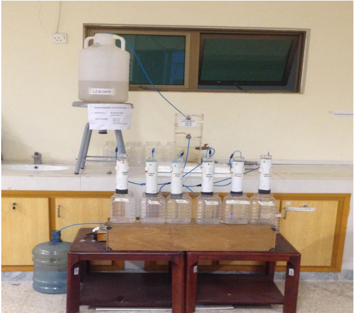
Figure 5 : Column adsorption setup installed in Air, Noise and Solid Waste Laboratory
