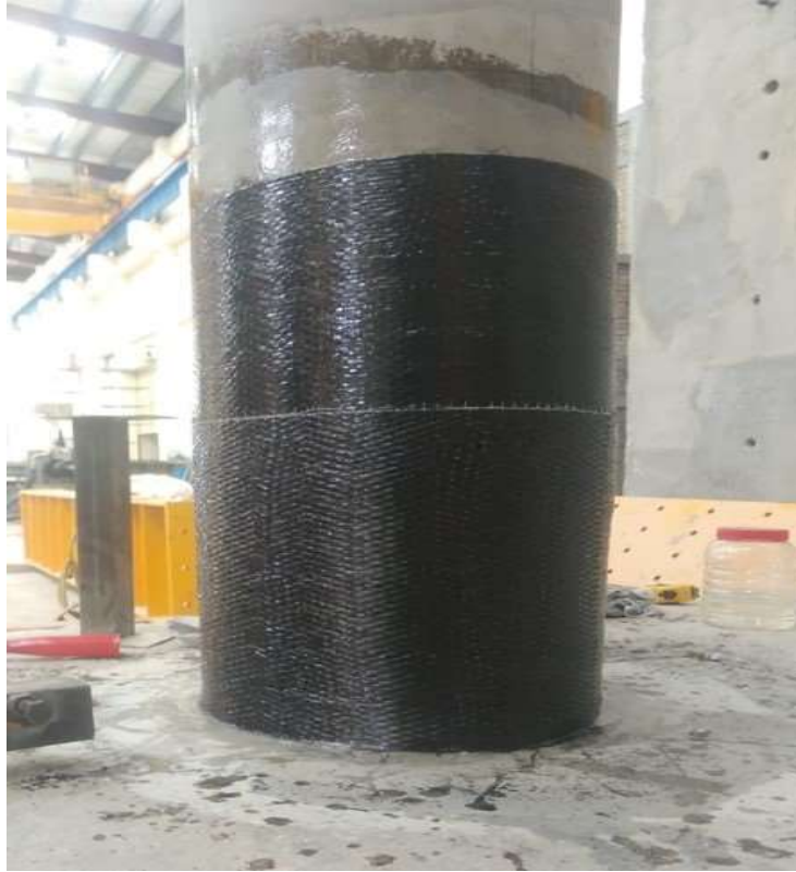
Figure 4. 8: Retrofitted specimen with two layers of CFRP jackets at hinge location.
