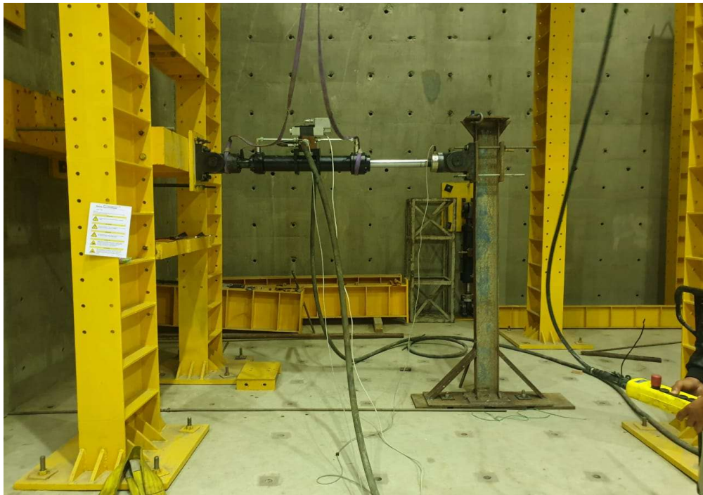
Figure 3.3: Experimental setup for quasi-static cyclic loading test on trial steel column
