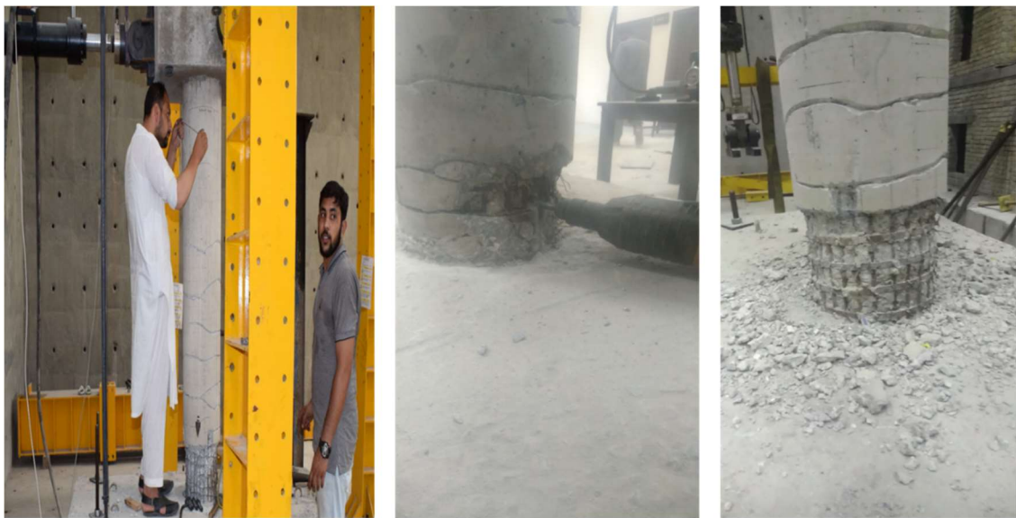
a) Bring column to zero position b) Removal of disintegrated concrete c) Adjusted pre-bent metal strips
