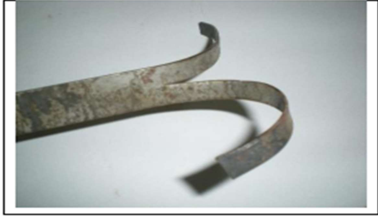
Figure 4.4: Pre-bent metal strips as a transverse reinforcement.
