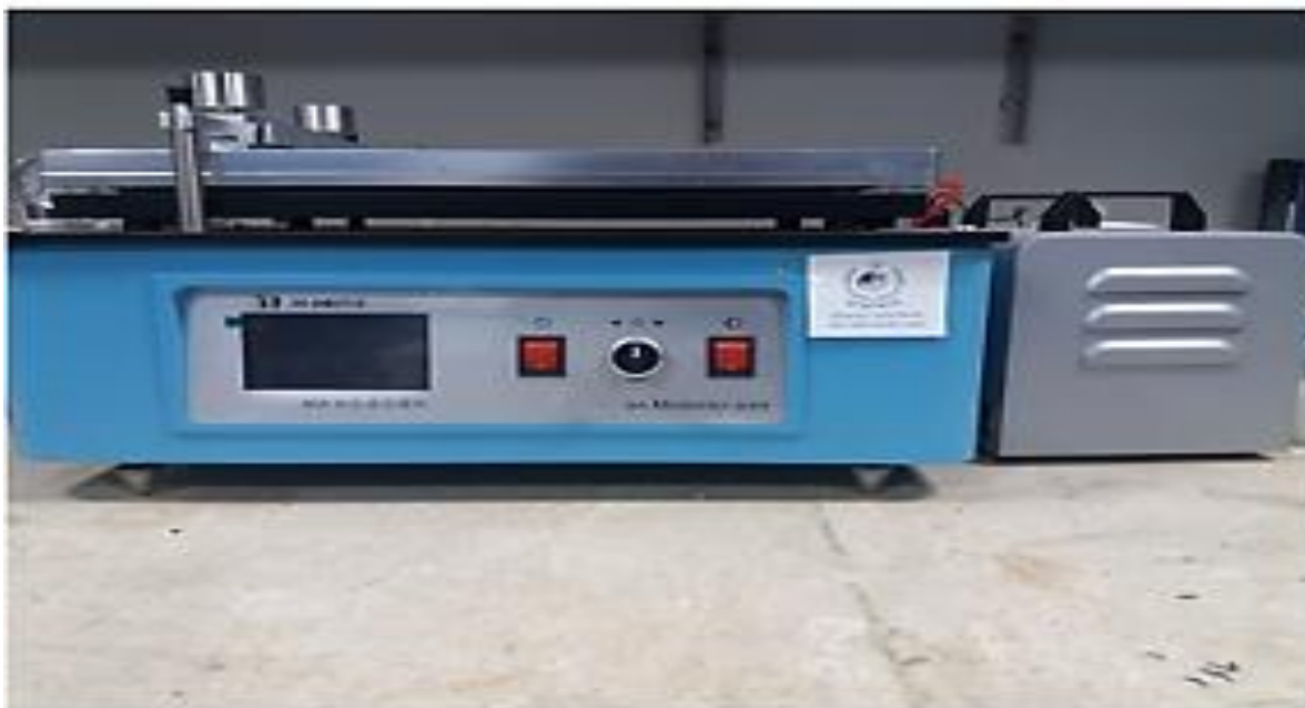
Figure 3.1 Polymer membrane manufacture appliance (Automatic Film Coater)
