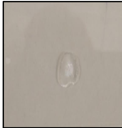
Figure 2: Positive Catalase test showing the emission of oxygen gas.
