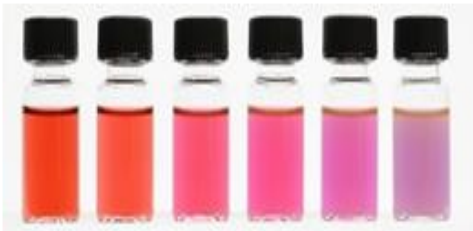
Figure 2.5: Colors of various sized monodispersed gold nanoparticles [42].
