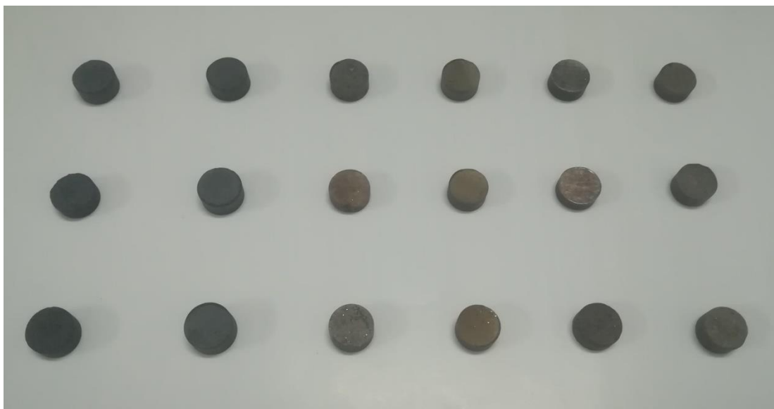
Figure 3.4: Six sets of samples after sintering
