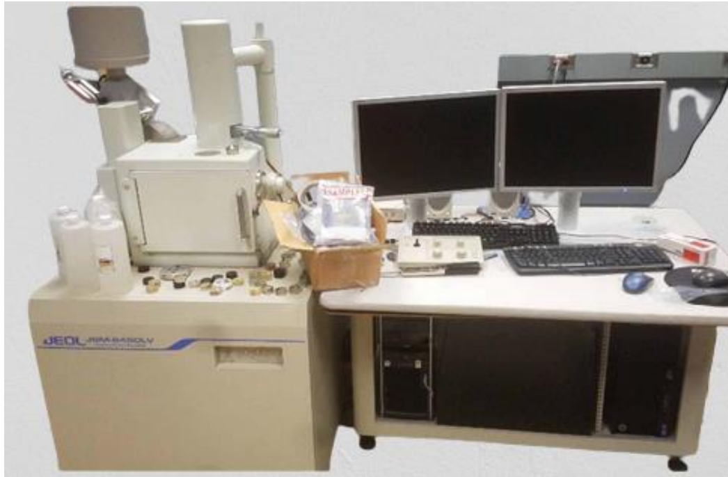
Figure 3.5 Scanning Electron Microscope Jeol 6490 LV [11]
