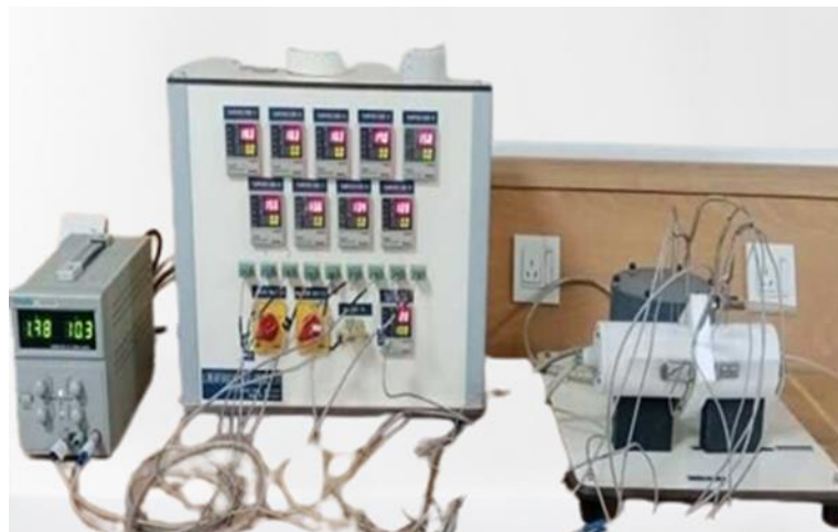
Figure 4.15 Thermal Conductivity Meter (I.S.T Islamabad)
