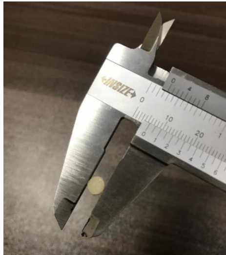
Figure 16: Measuring the diameter of composite disc
