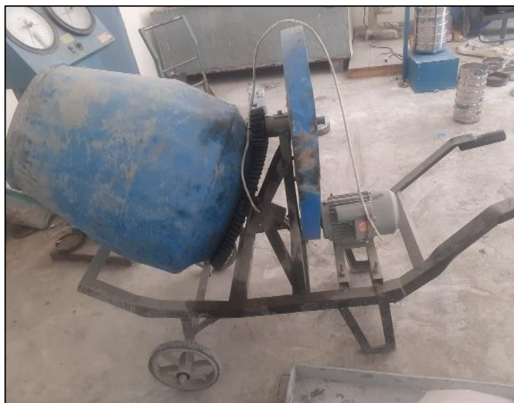
Figure 20: Concrete mixer machine
