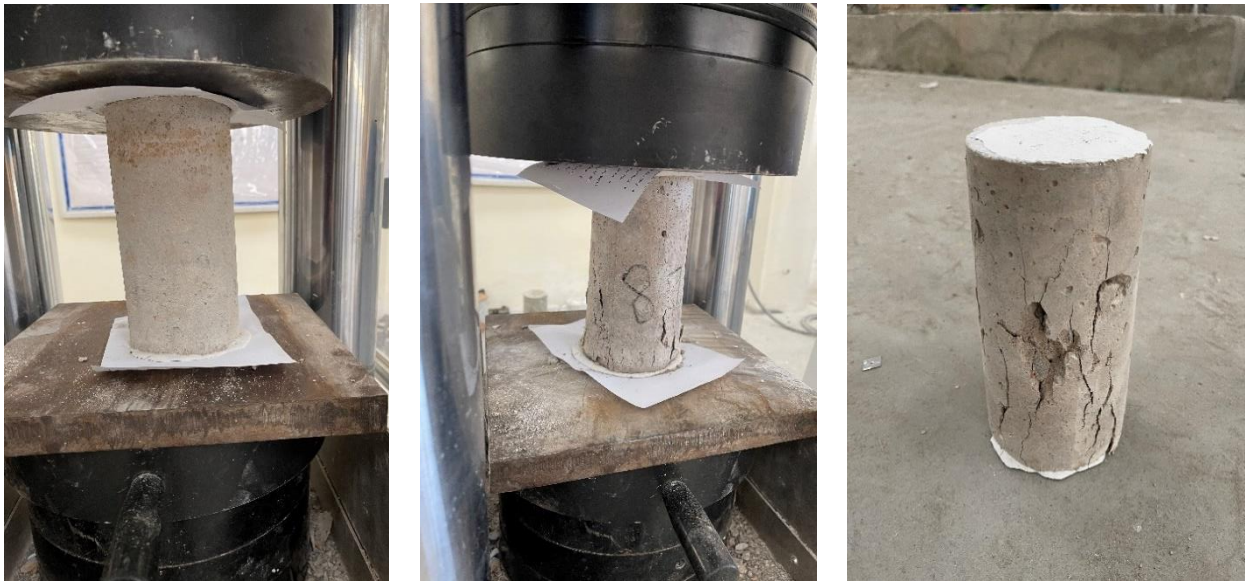
Figure 3.8 Concrete Compressive Apparatus and Failure Pattern
