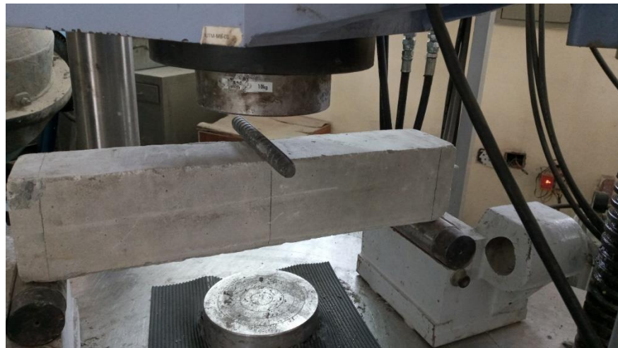
Figure 4.7 Flexural test of Beam
