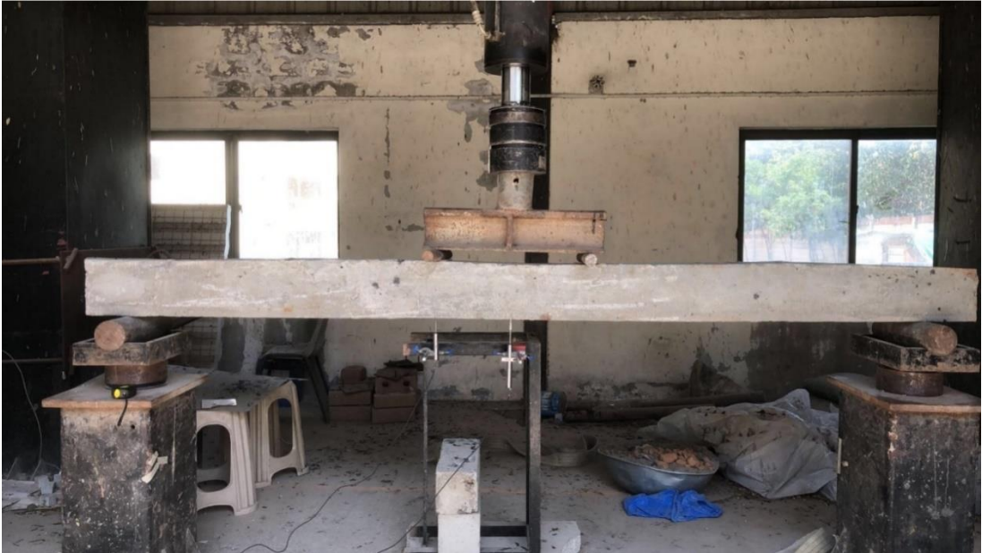
Figure 4.10 Experimental setup of RCC Beams
