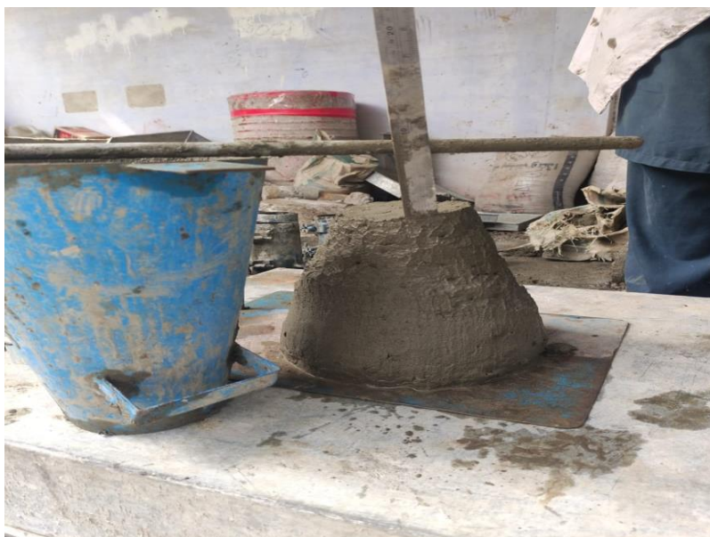
Figure 4.1 Control Mix Slump
