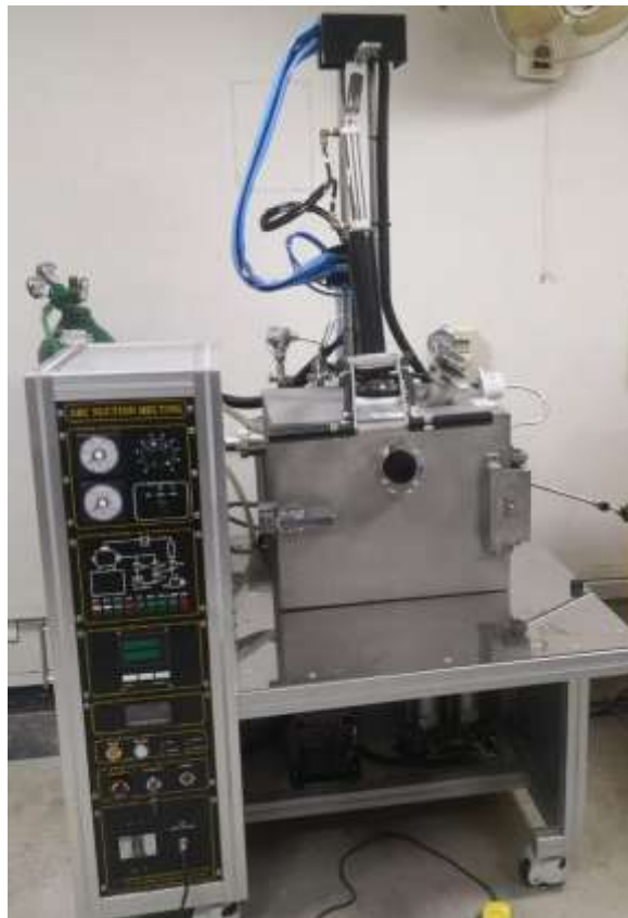
Figure 3-1 Vacuum arc suction melting furnace in SCME, NUST
