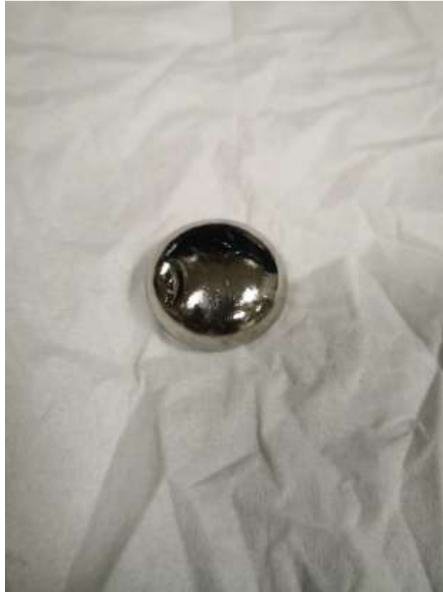
Figure 3-2 Button shape metallic sample formed in Vacuum arc suction melting furnace present in SCME, NUST.
