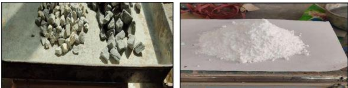
Figure 3.10 Shows Sample For Soundness Test
