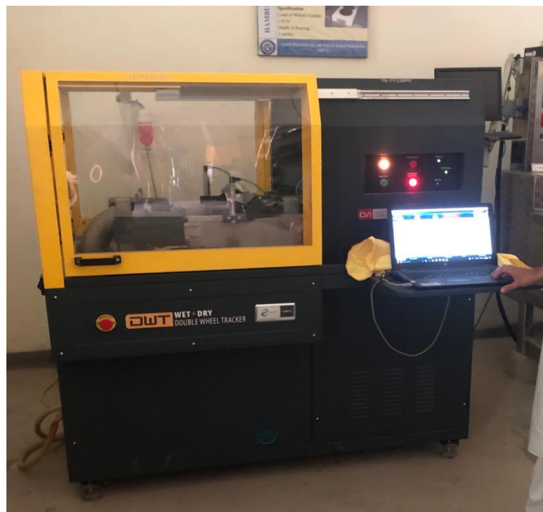
Figure 3.25 DWT for Rutting test
