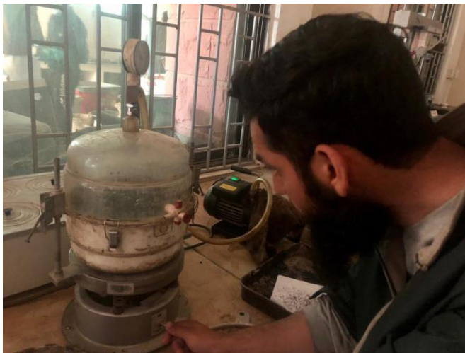
Figure 3.20 Apparatus For Gmm And Prepared Samples For Gmm
