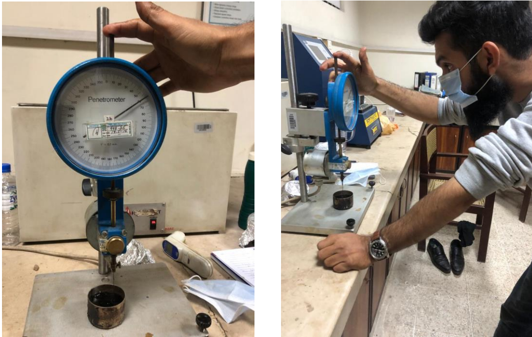
Figure 3.11 Shows Penetration Test Apparatus
