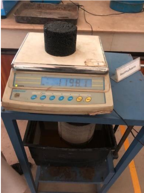
Figure 3.21 Gmb Test Apparatus And Prepared Samples In Water Bath
