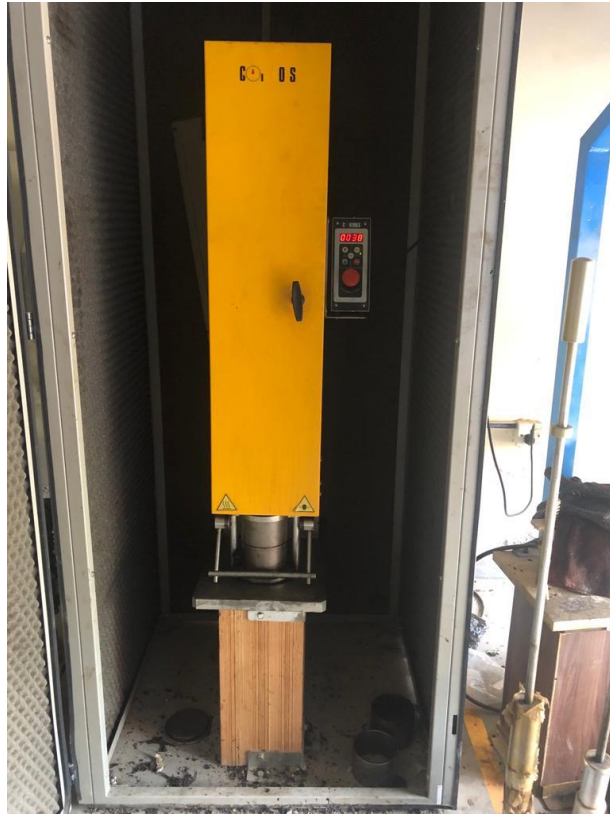
Figure 3.18 Automatic Compactor for samples
