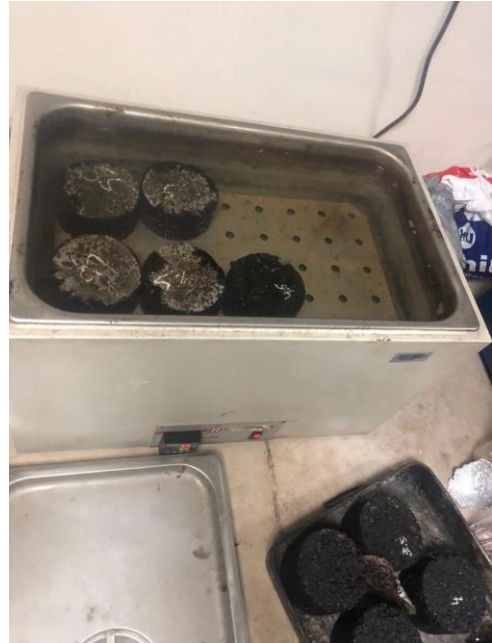
Figure 3.21 Gmb Test Apparatus And Prepared Samples In Water Bath
