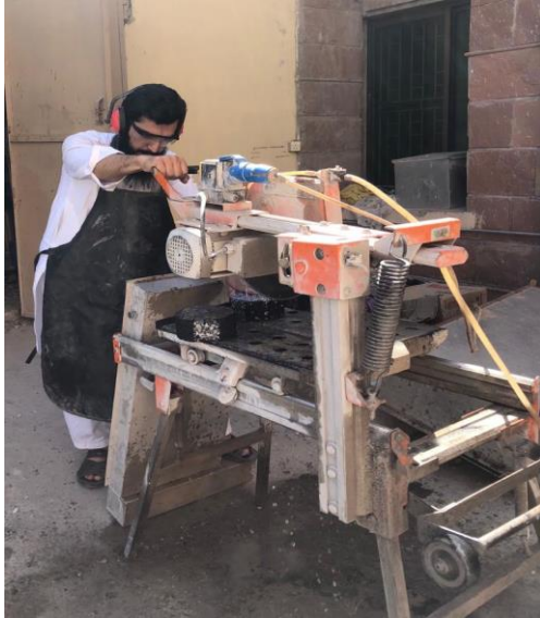
Figure 3.24 Saw Cutter And Samples For DWT
