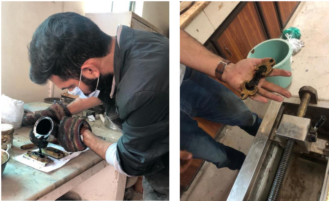
Figure 3.13 Shows Sample Preparation For Ductility Test And Test Apparatus
