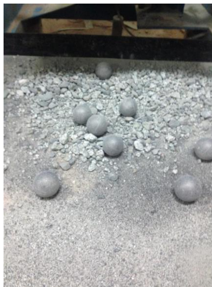
Figure 3.5 Tested Aggregate Sample in LA Apparatus
