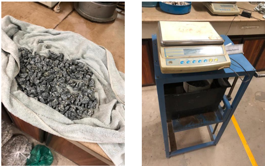
Figure 3.8 Shows Saturated sample and Test Apparatus
