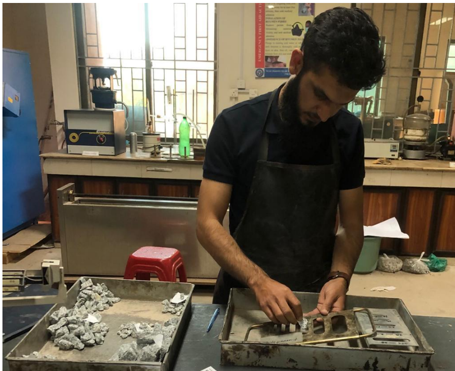
Figure 3.4 Shows Flakiness index Apparatus
