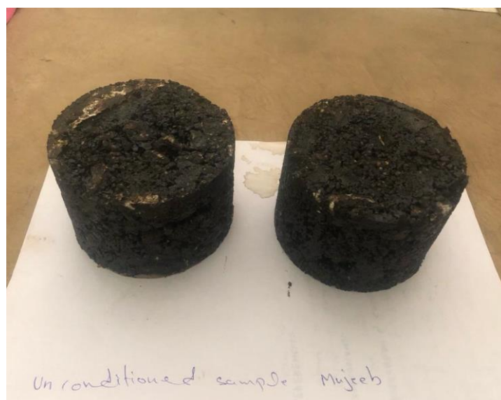
Figure 3.28 Prepared Unconditioned Sample for UTM
