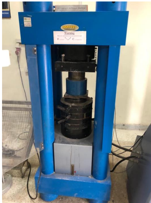
Figure 3.9 Shows Compressive Testing Machine And Steel Cylinder
