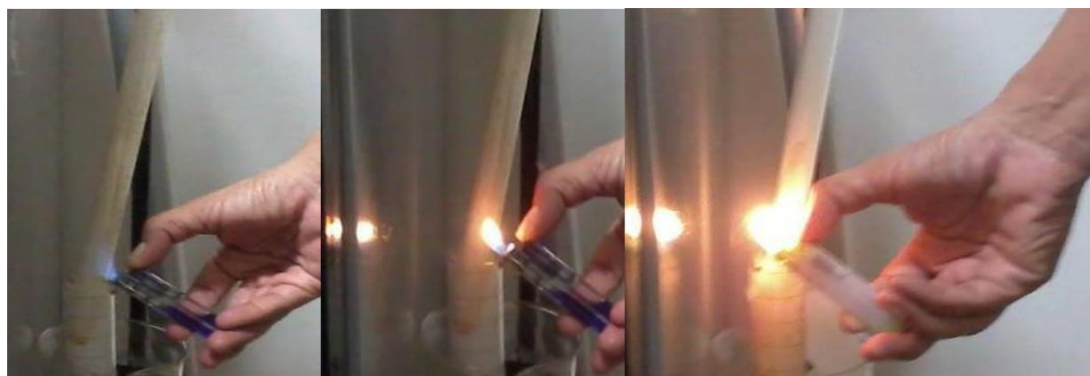
Fig. 4.8: Flame test of presence of hydrogen rich gas
