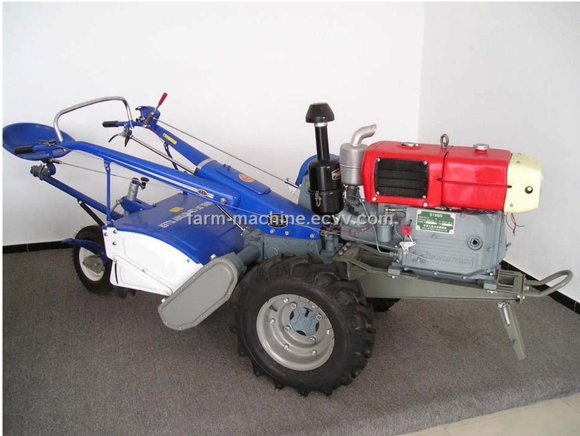
Figure 2- Walking Tractor DF-12
