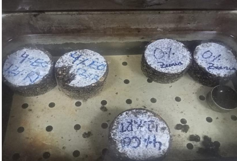
Figure 3-20 Sample for IDT and moisture susceptibility test in the oven for 24hrs (conditioned sample)
