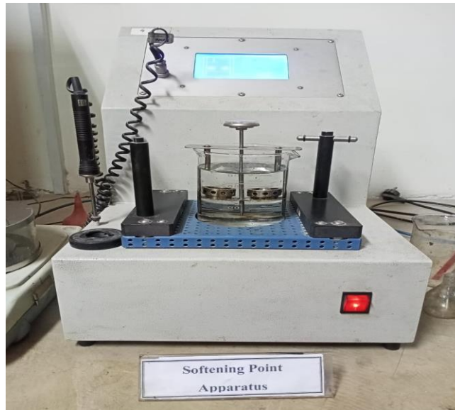
Figure 3-9 Softening Point test apparatus (ring and ball assembly)
