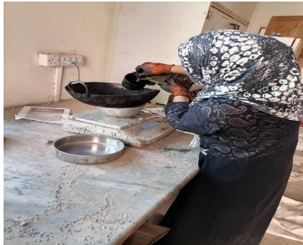
Figure 3-16 Bitumen preparation before mix design
