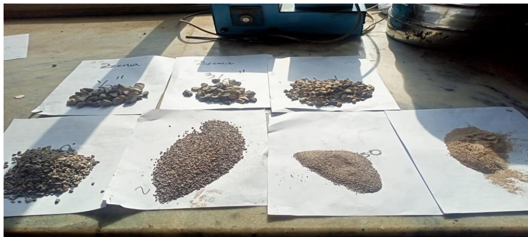
Figure 3-15 Sample aggregates for asphalt
