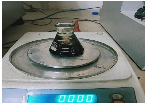
Figure 3-13 Pycnometer for finding the specific gravity of the sample
