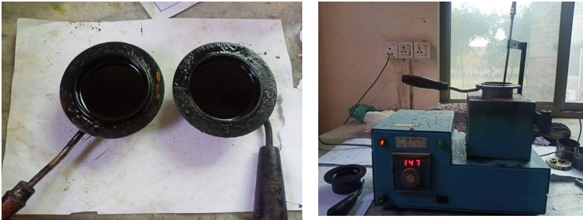
Figure 3-12 Flash and fire apparatus
