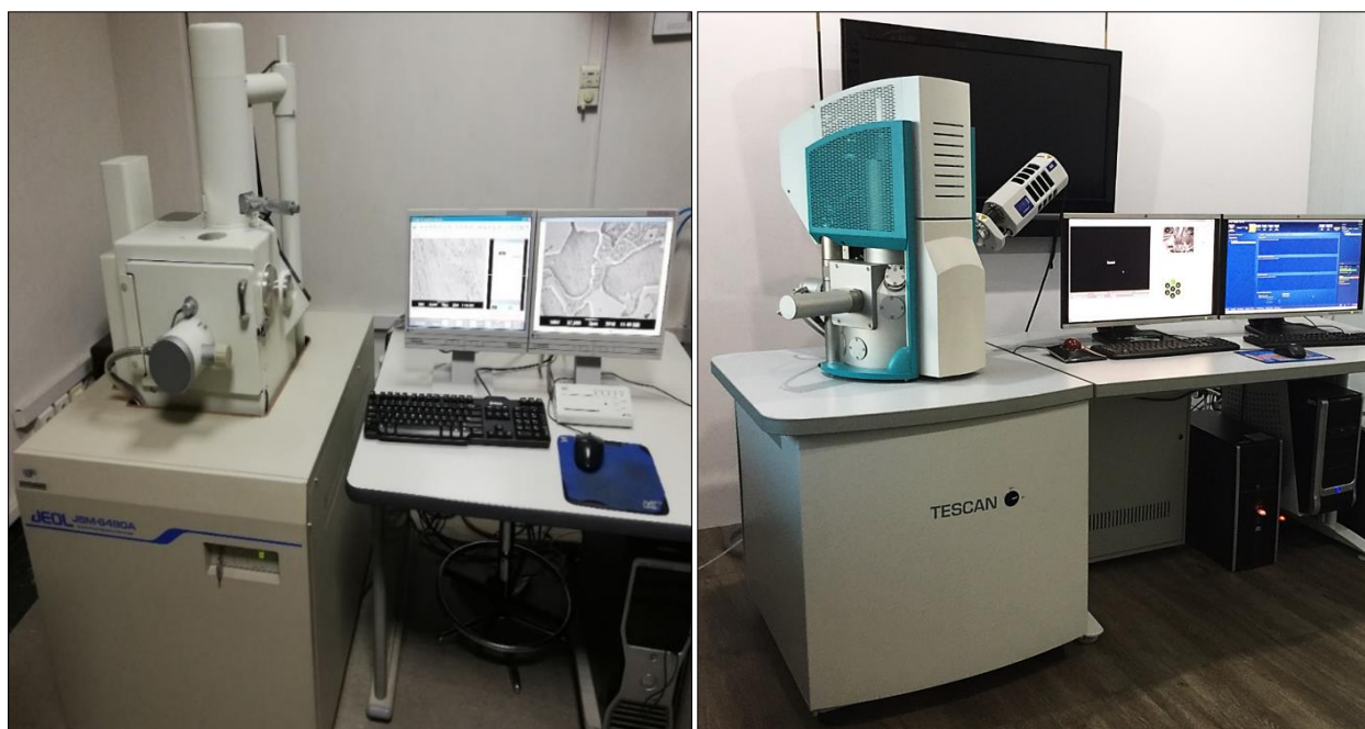
Figure 3-1 Scanning electron microscope equipped with EDS at SCME (left) and at USPCASE, (right) NUST.
