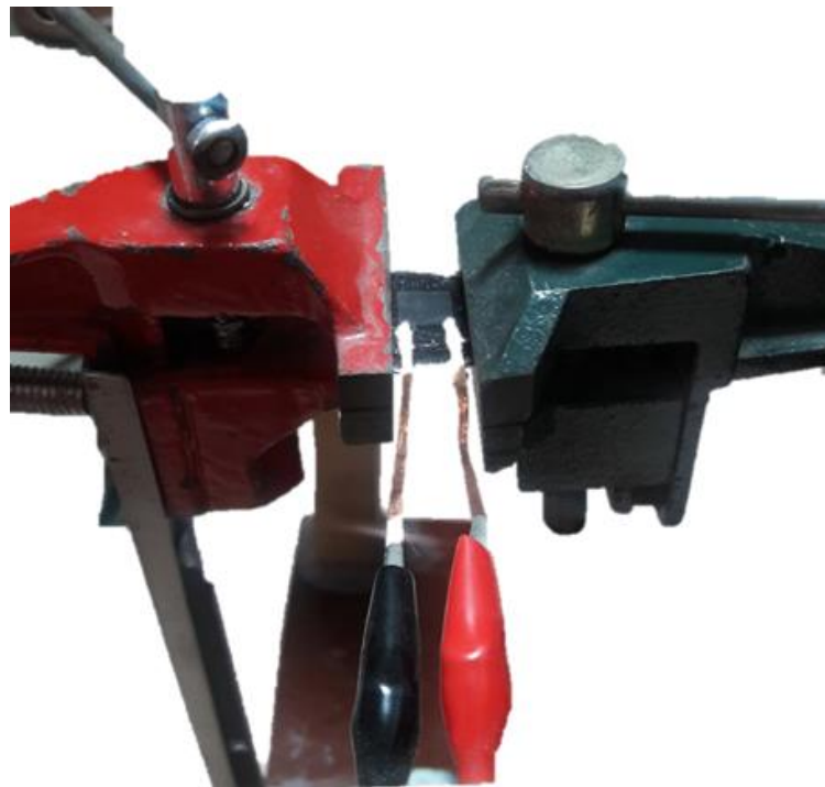
Fig 22: Clamps to hold the device that can move up, down and, twist on either side.
