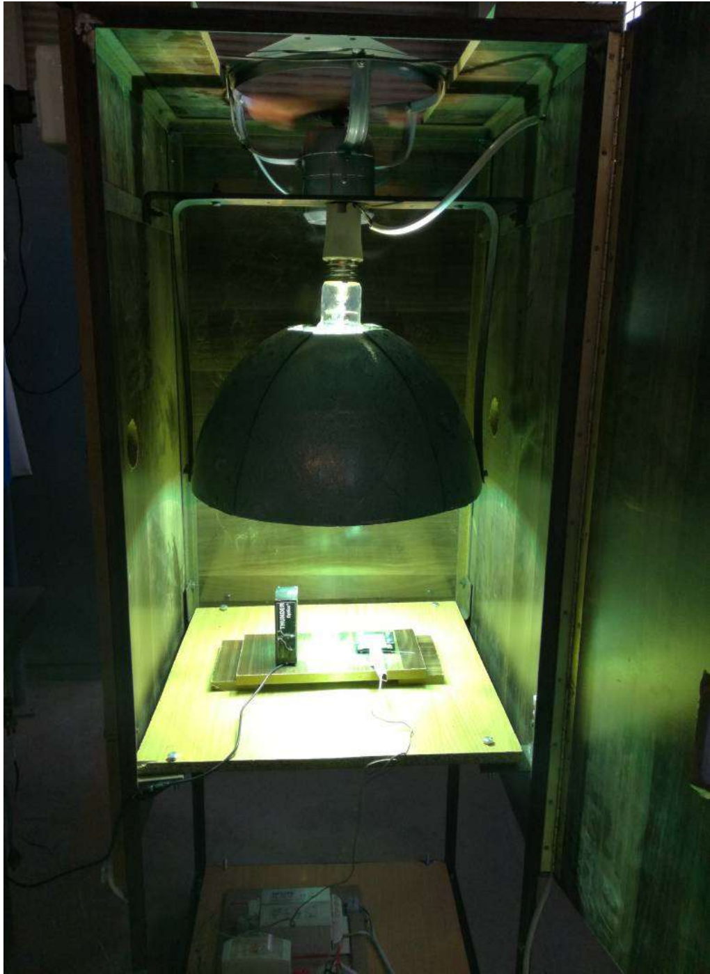
Figure 23: Fabricated solar simulator
