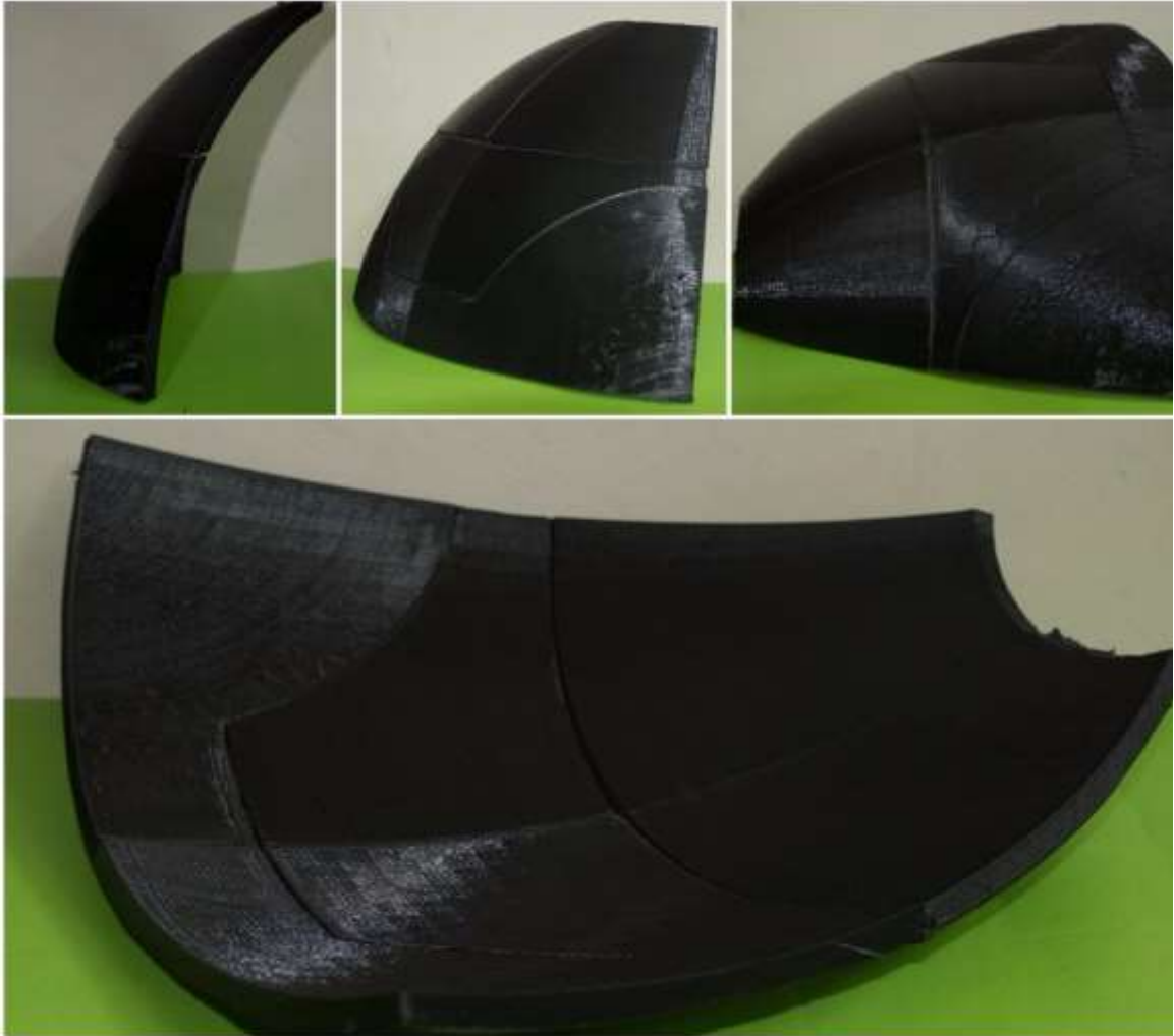
Figure 15: 3D printed mold for reflector(Quarter)
