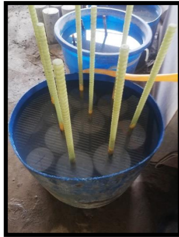
Figure 3. 3 Curing of Concrete Cylinders in Seawater
