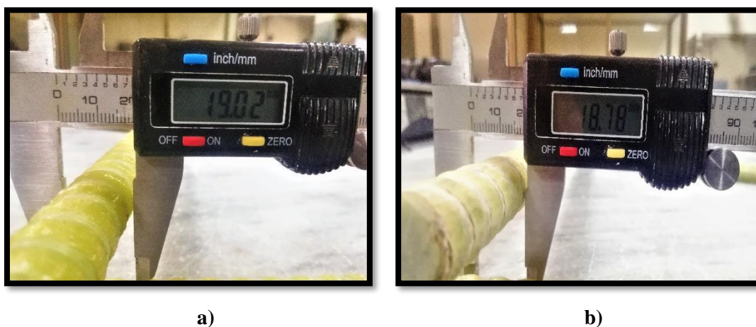
Figure 4. 11 Reduction in the Bar Diameter a) Before Pull-out test b) After Pull-out Test
