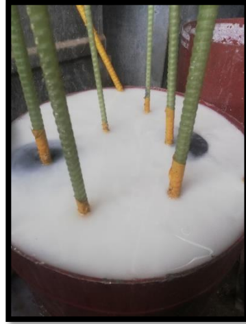
Figure 3. 4 Curing of Concrete Cylinders in Alkaline Solution
