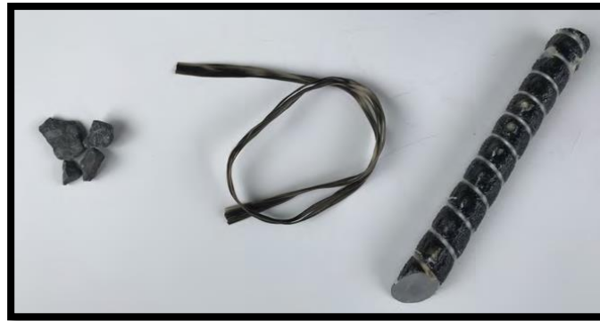
Figure 2. 2 Basalt FRP bar Manufacturing Steps
