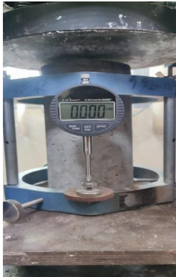
Figure 11: Test Setup for Modulus of Elasticity
