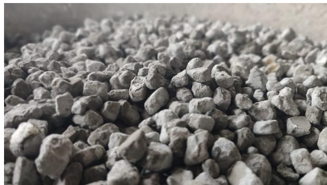
Figure 4: Cement coated PU foam aggregates
