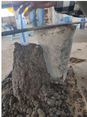
Figure 8: Measurement of Slump Value
