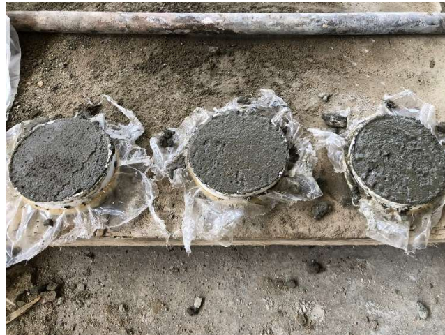
Fig. 13: Discs of concrete for thermal conductivity test
