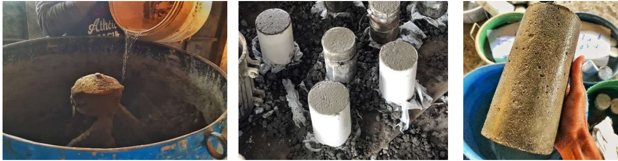
Fig. 12: Process of casting PCM incorporated concrete cylinders
