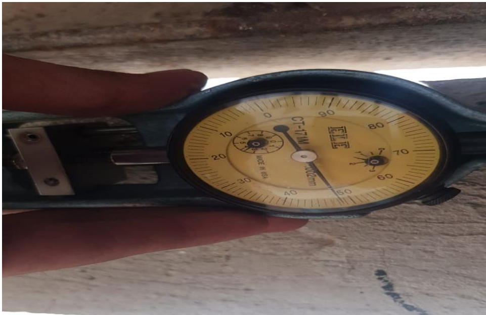
Figure 24: Strain Measurements Using Demec Gauge
