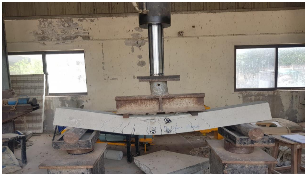
Figure 25:Cracking Induced in Beam due to Loading
