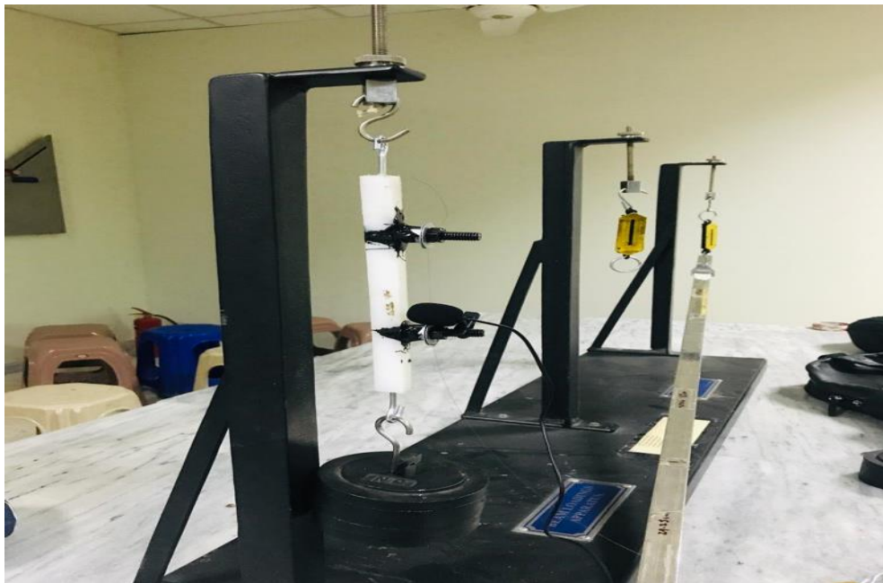
Figure 22: Loading Applied on Nylon Bar to Induce Applied Strain
