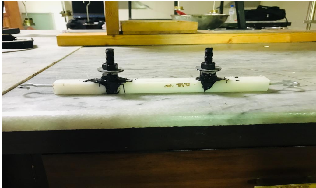
Figure 21: Calibration Gauge Setup on Nylon Bar
