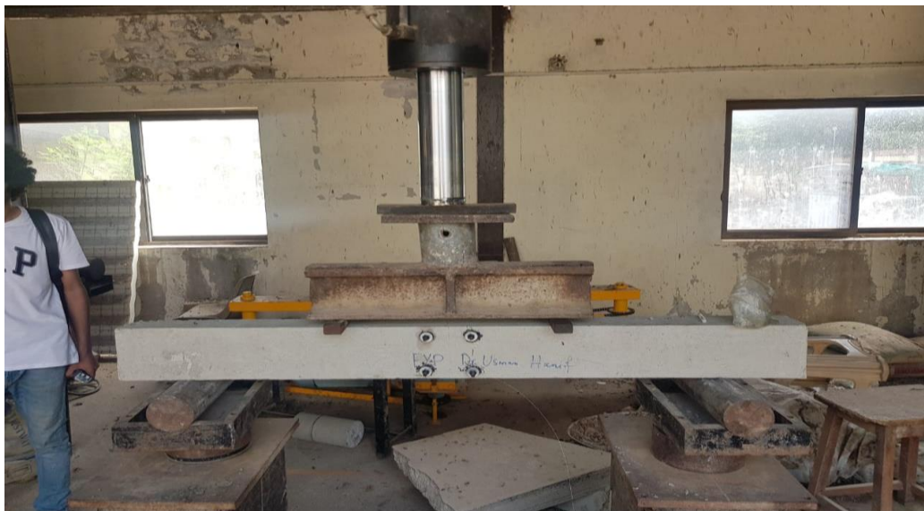
Figure 23: Beam Placed on Loading Rig to Induce Damage
