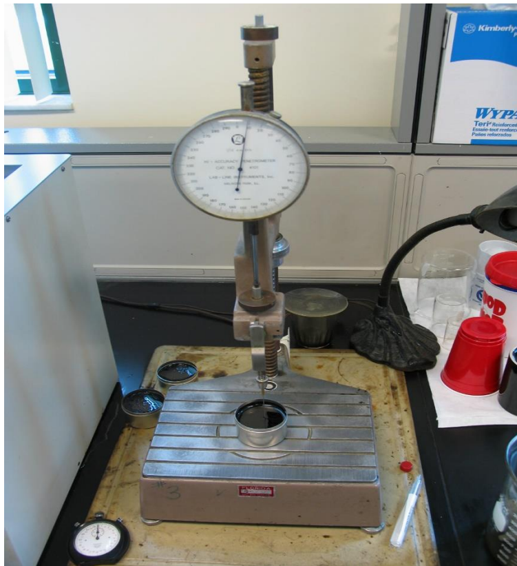
Fig 3.6.1(Penetration Test Equipment)
