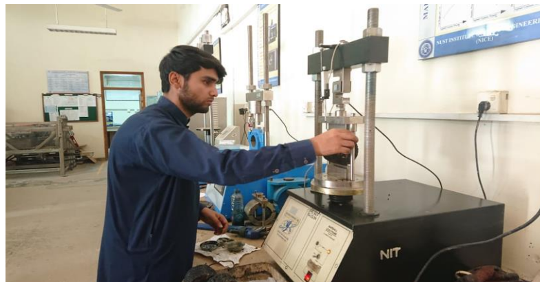
Figure 3.15 Performing ITS Test
