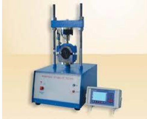
Fig 3.10 (Marshall Stability and Flow Apparatus)
