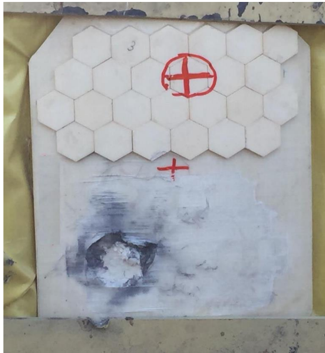
Figure 46 : Ballistic panel after first shot
