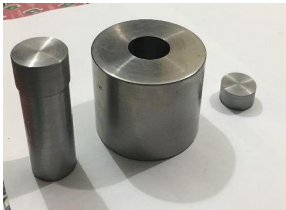
Figure 14 : Circular die used to press powders to green compacts
