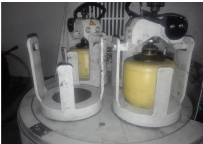
Figure 12 : A planetary ball mill used to mill/mix powder samples
