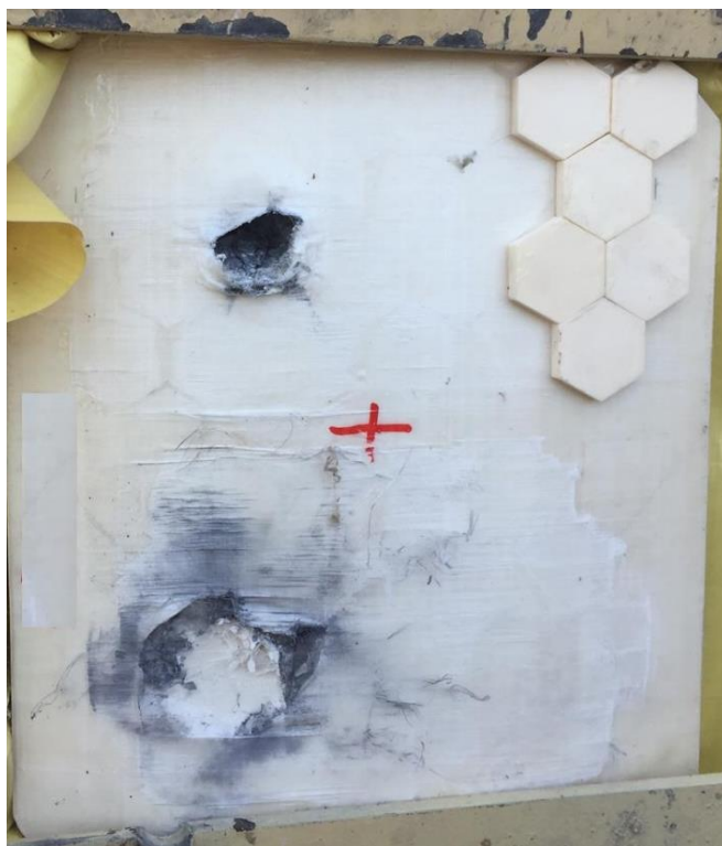
Figure 47 : Ballistic panel after second shot
