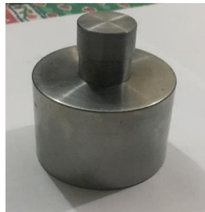
Figure 14 : Circular die used to press powders to green compacts
