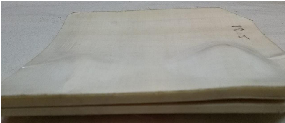
Figure 49: Side view of the panel showing trauma after testing
