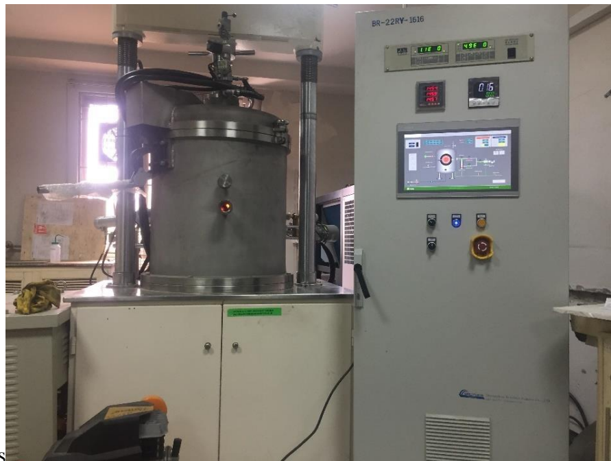
Figure 16 : High temperature furnace used to sinter the samples
