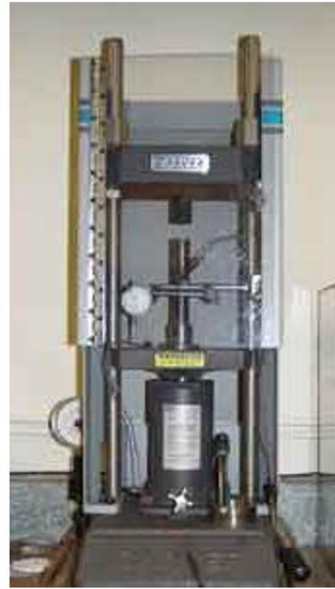
Figure 13 : A manual hydraulic press used to make green compacts
