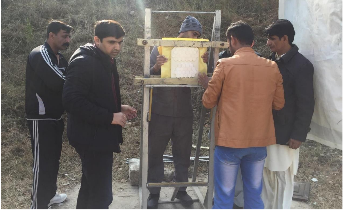
Figure 45 : Fixation of ballistic panel for testing
