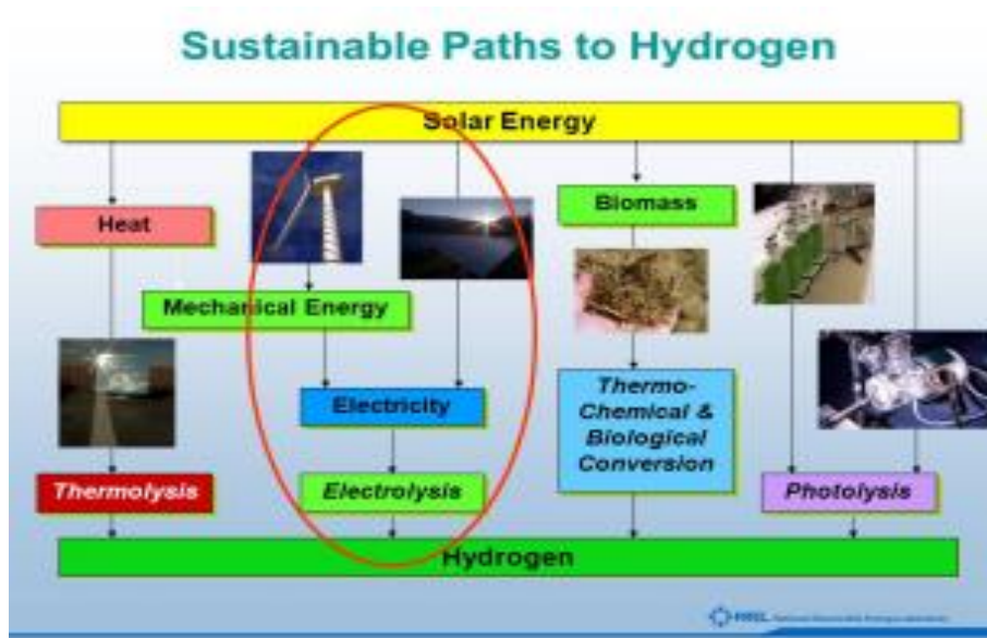
Figure 1- 3 Sustainable pathways for hydrogen generation from solar energy [16]
