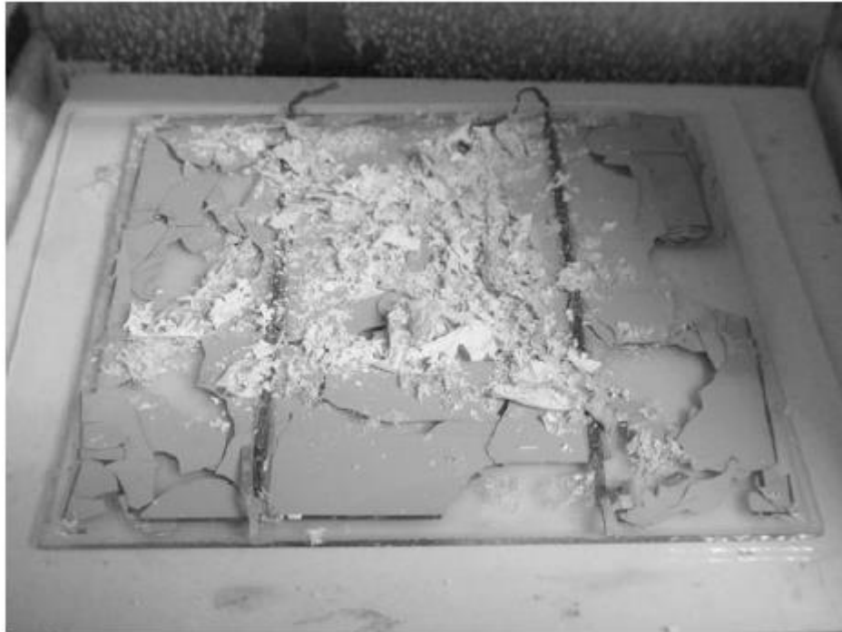
Figure 12: Remaining components of Si module after thermal treatment.
