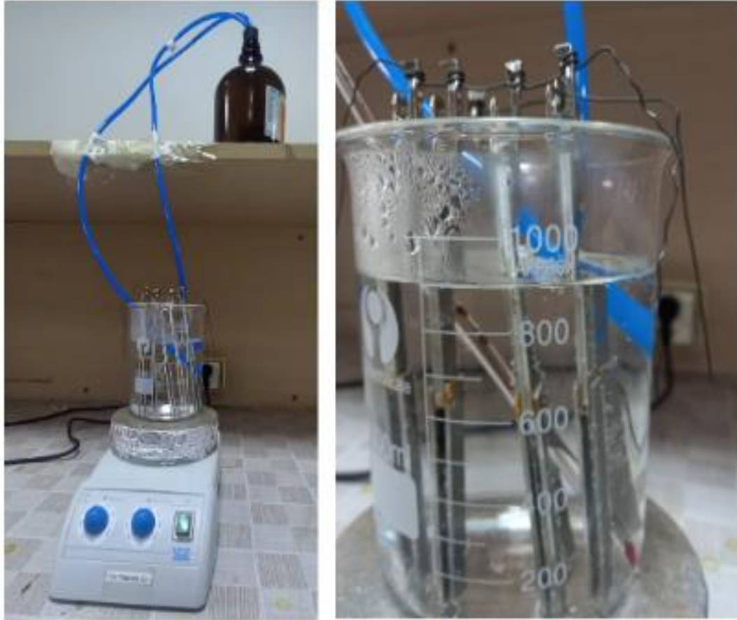
Figure 4.1- 3 Hydrothermal Aging setup
