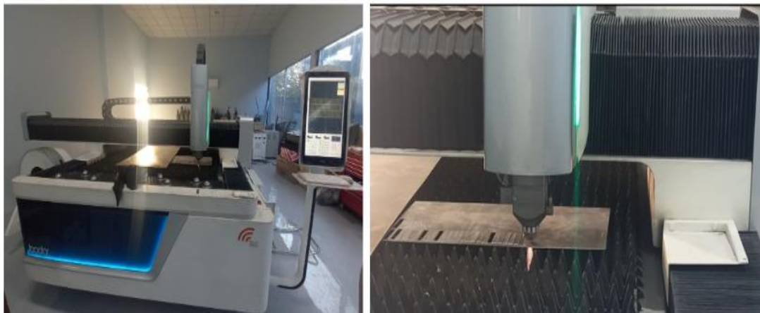
Figure 3.1- 2 Laser Cutting of EN AW-6061 T6 Sheet
