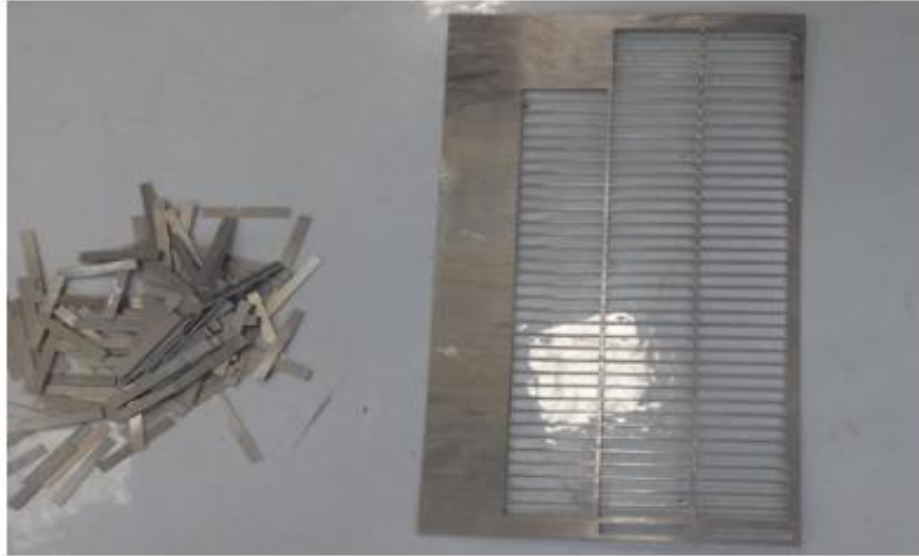
Figure 3.1- 3 EN AW-6061-T6 Sheet after Laser cutting
