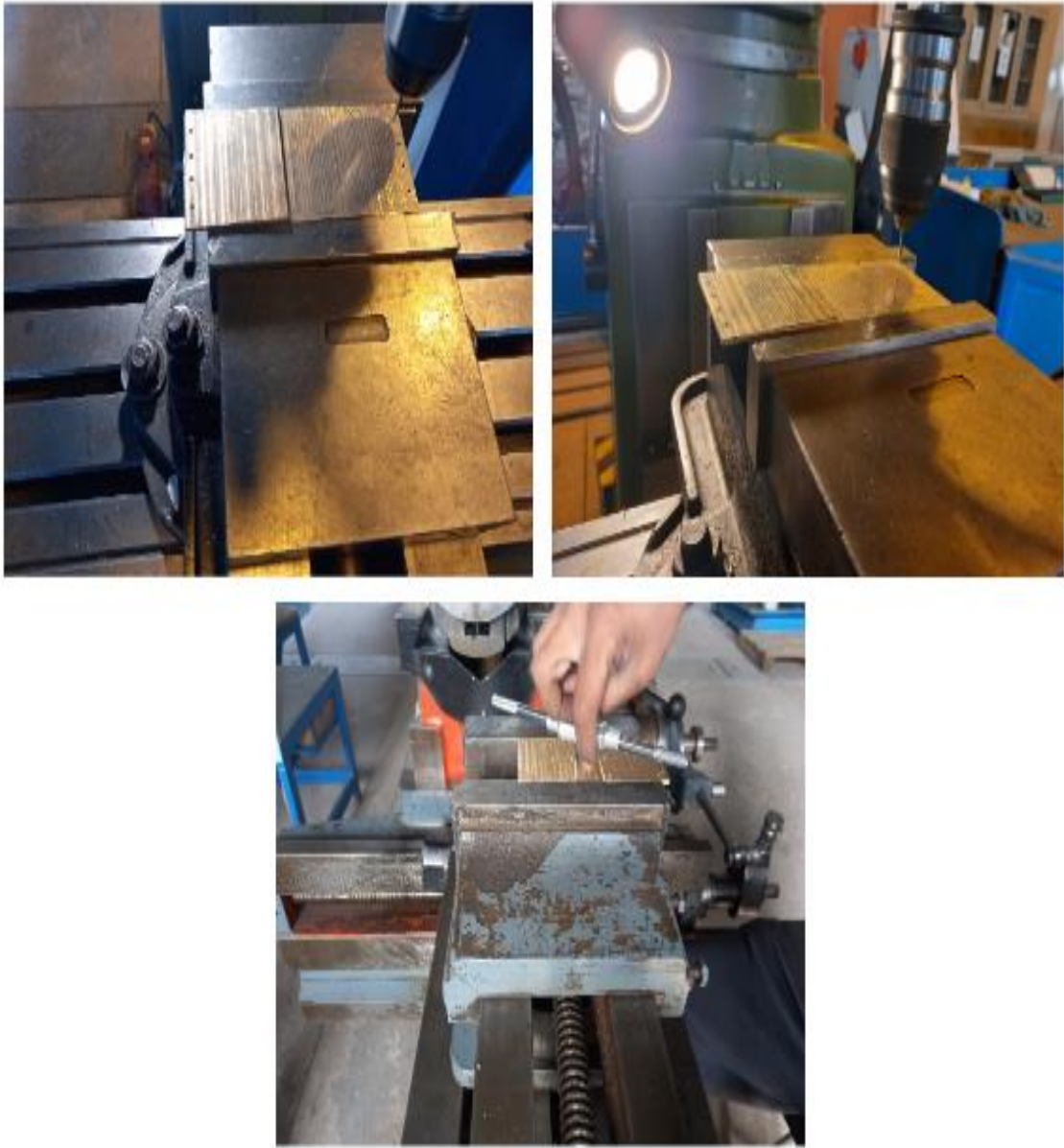
Figure 3.3- 7 M3 screw holes drilling and tapping
