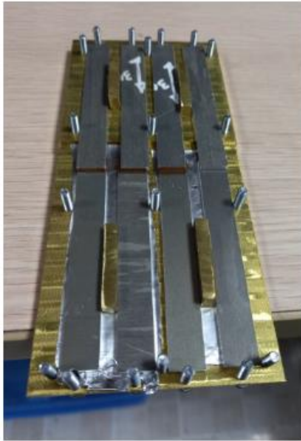
Figure 3.3- 1 Bonding tool for Adhesive Joints
