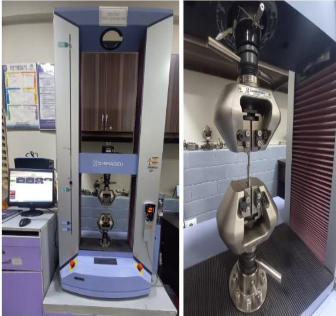
Figure 4.1- 2 Single lap joint shear test setup
