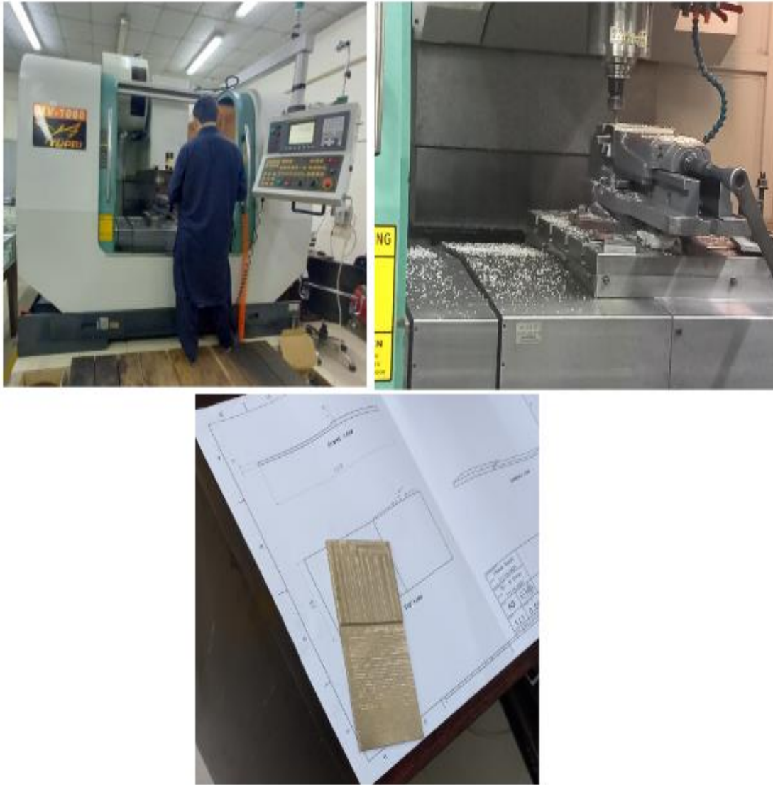
Figure 3.3- 5 Manufacturing of Bonding tool by CNC milling machine
