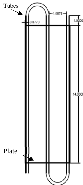
Figure 3.5 Panel front view drawn using AutoCAD
