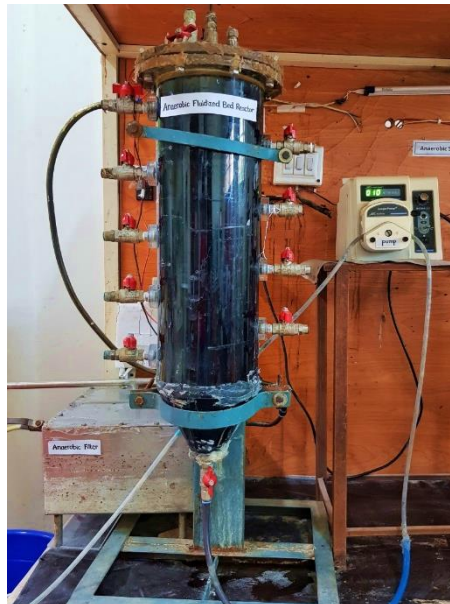
Figure 0.7 Lab Scale Setup of AFBR-AF
