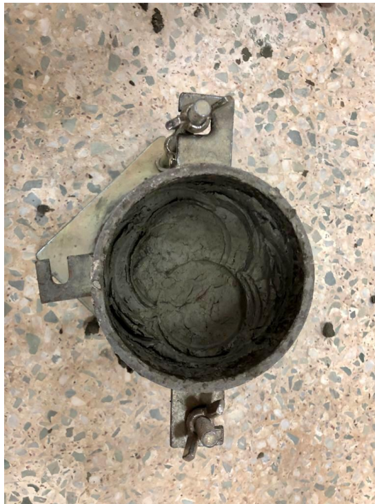
Figure 5 Proctor Test being performed
