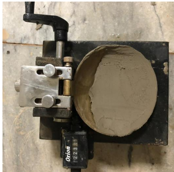
Figure 3 Liquid Limit test being performed
