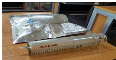
Figure 3.11 Syringe and Gas Collection Bag
