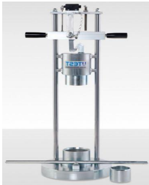
Figure 3.4 Aggregate Impact Value Apparatus
