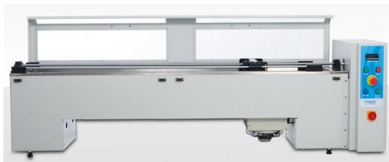
Figure 3.9 Ductility Test of Bitumen Apparatus
