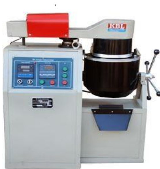
Figure 3.11 Mixer for producing Asphalt Mixture
