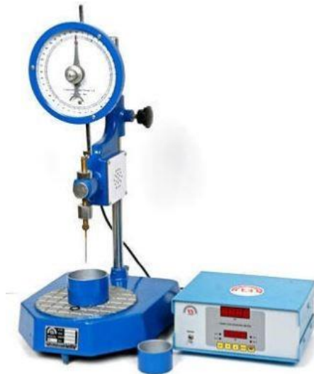
Figure 3.7 Bitumen Penetration Test Apparatus
