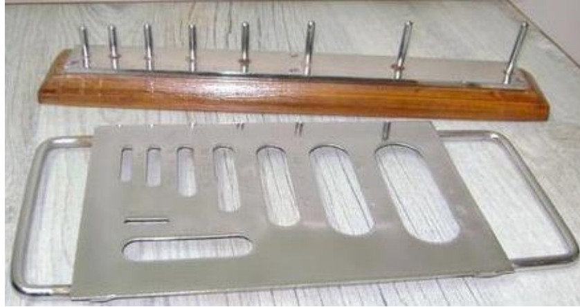
Figure 3.5 Flakiness and Elongation Test Apparatus
