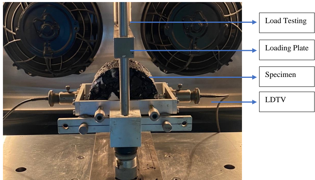
Figure 3.21 Assembly of Resilient Modulus Test
