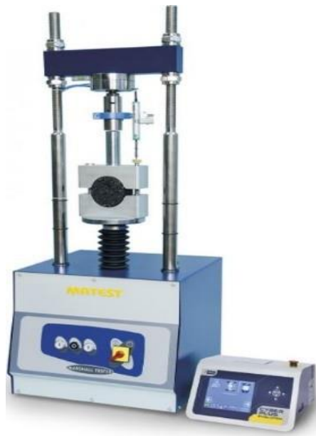
Figure 3.14 Marshall Test Machine
