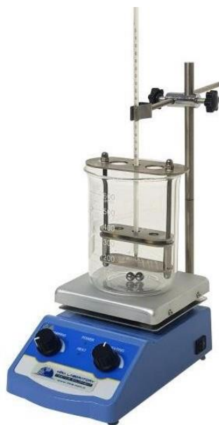
Figure 3.8 Ring and Ball Apparatus for Softening Point of Binder
