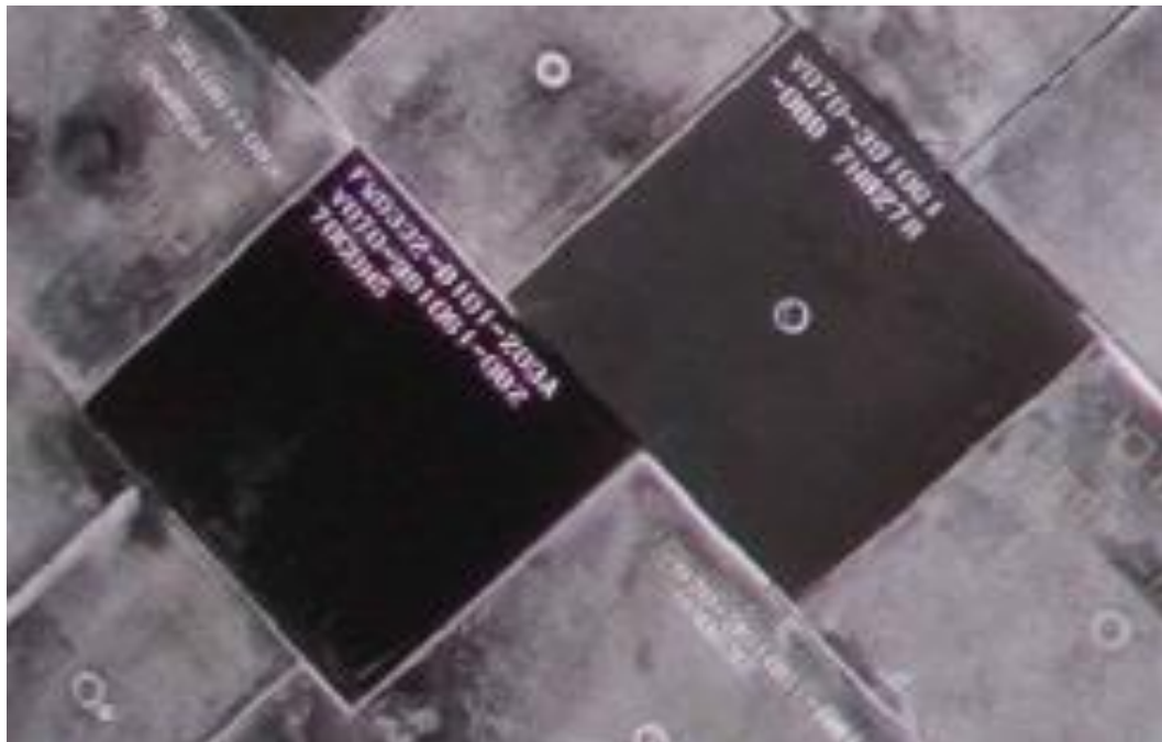
Figure 7 Alumina Enhanced Thermal Barrier (AETB) tile [21]
