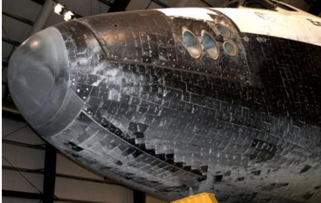
Figure 3 Application of TPS at nose cap and belly of space shuttle [17]
