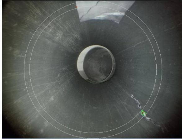
Figure 15 Region of Interest of the robot is captured between two circular rings
