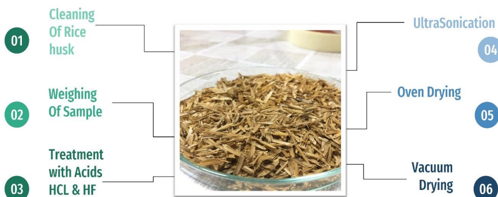
Figure 4: Elaboration of various steps involved in washing of the as obtained rice husk samples.
