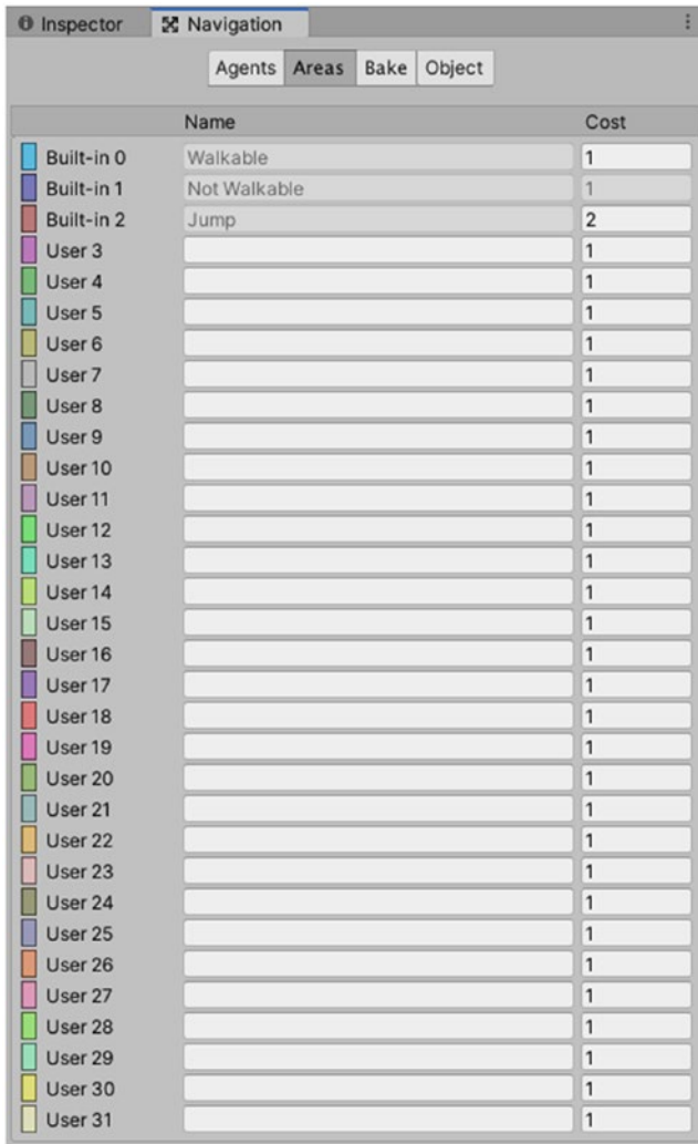
Figure 4-10. The Areas tab in the Navigation panel allows you to create different types of areas and assign different costs to them
