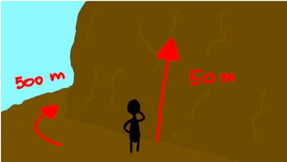
Figure 4-3. A pathfinding algorithm that doesn't take into account the costs of climbing 50 m of rocky wall compared to those of walking 500 m on a comfortable path, might take the wrong decision judging which of the two paths is the best
