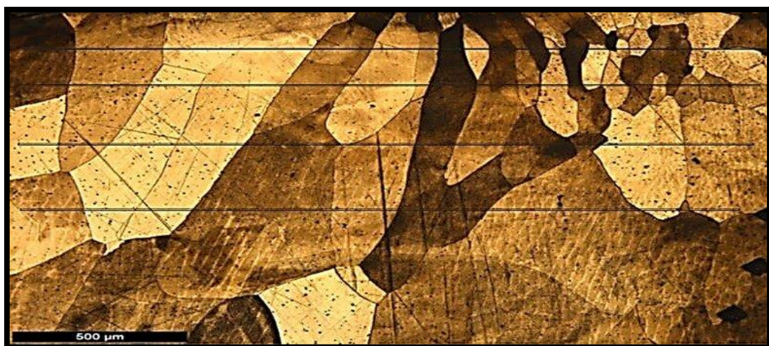
Figure 3.7: Linear Intercept method applied ion OM images for Grain size measurement
