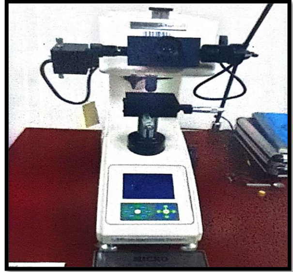
Figure 3.12:(left) Microhardness indents (right)Micro Vickers hardness tester at SCME, NUST
