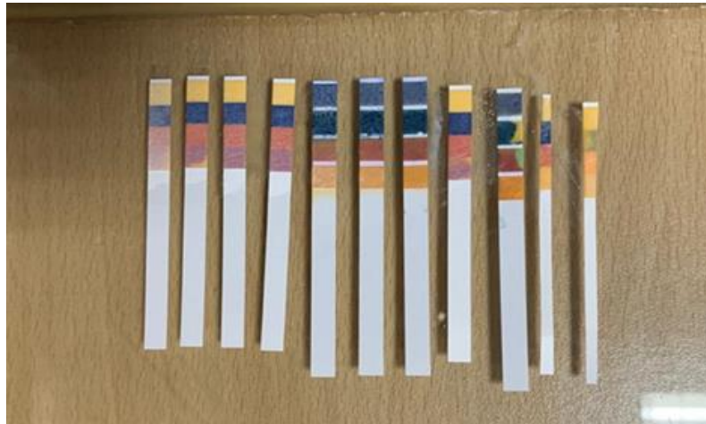
Figure 16 - pH Strips for each acid-addition interval
