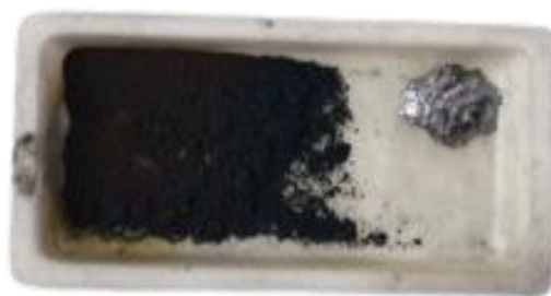
Fig. 5. Copper Selenide powder sample (left) with unreacted silvery mass of Selenium with impurities (right)
